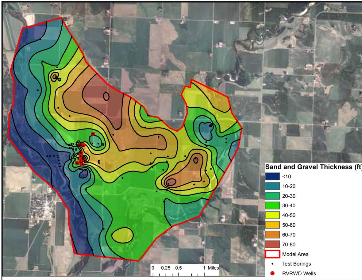
**Figure 7.** Isopach map showing the sand and gravel thickness for the Hudson aquifer.
