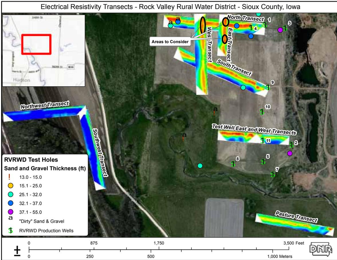
**Figure 6.** The geophysical (electrical resistivity) cross sectional results. Sand and gravel is indicated by the yellow and red zones, and silt and clay are indicated by the blue and green zones..
