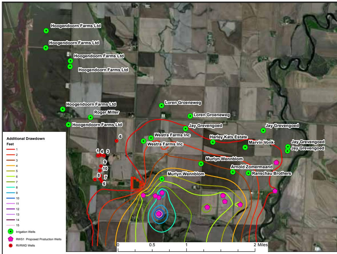
**Figure 13.** Simulated additional drawdown in feet caused by the proposed peak season pumping of the RWS #1 well field.
