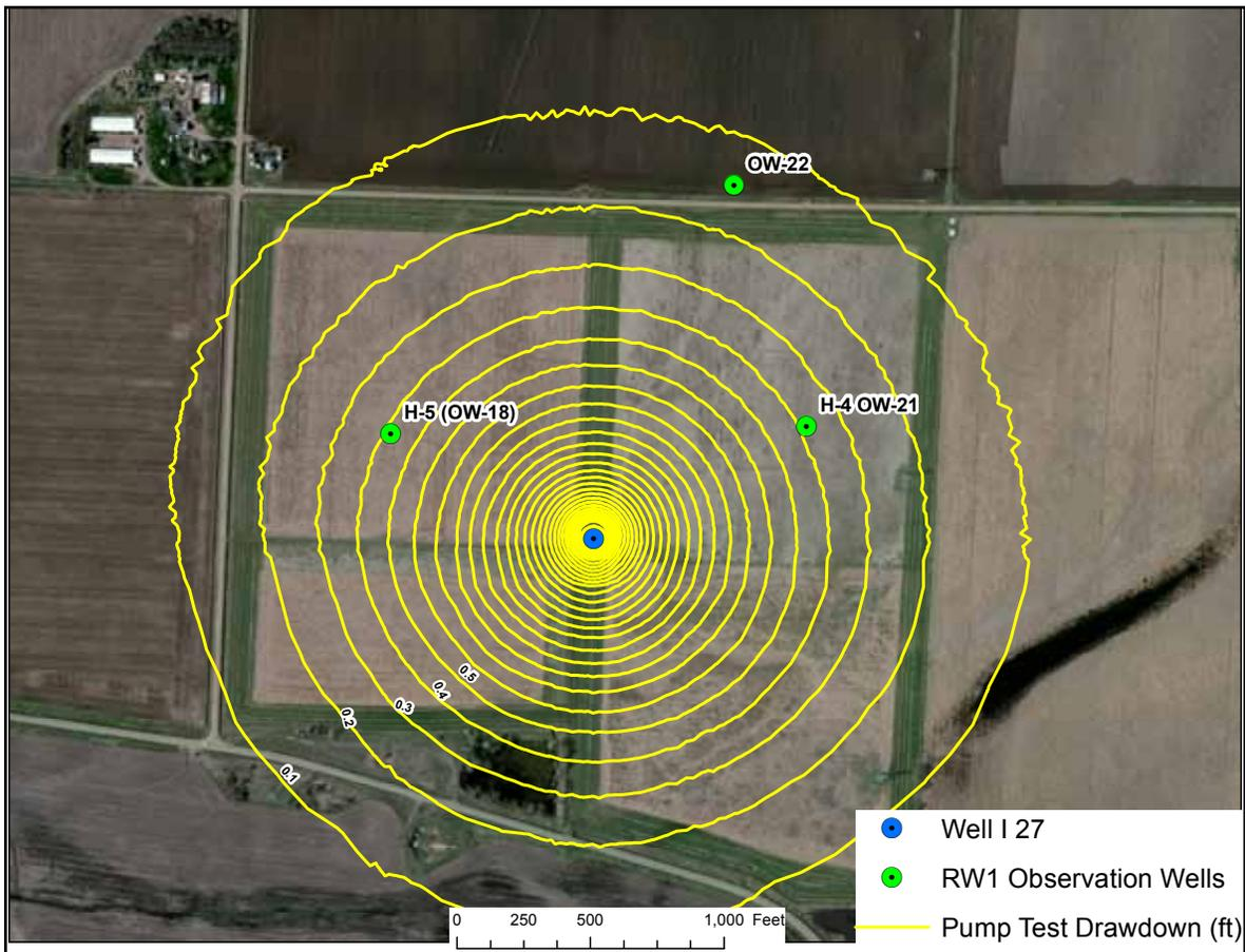
**Figure 9.** Simulated drawdown for the Rural Water System #1 well field pump test.
