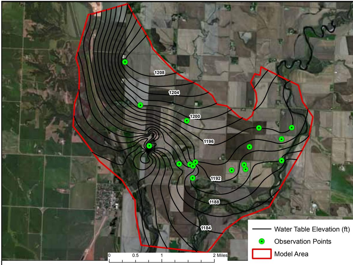
**Figure 4.** Static water table elevation map of the Hudson aquifer based on 2013 water levels.
