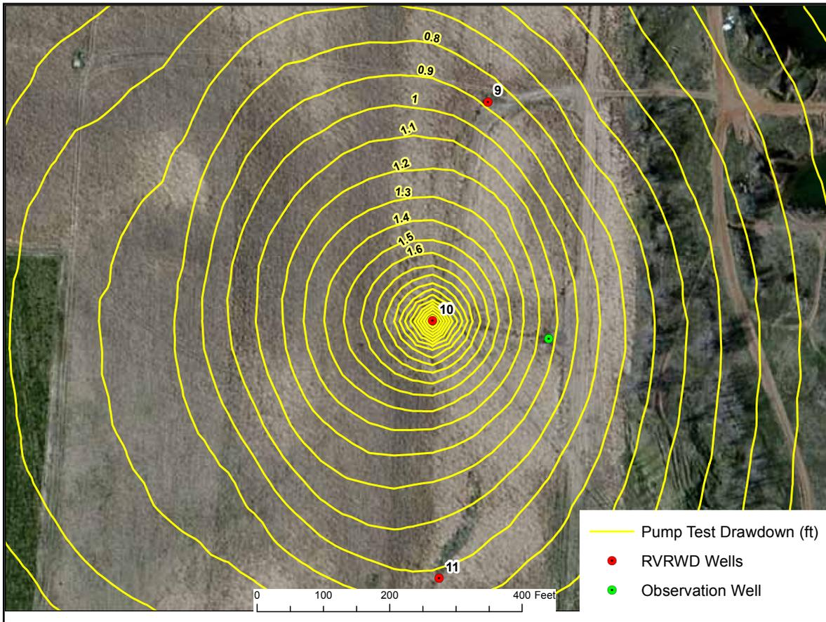
**Figure 8.** Simulated drawdown for the RVRWD (Well 10) pump test.
