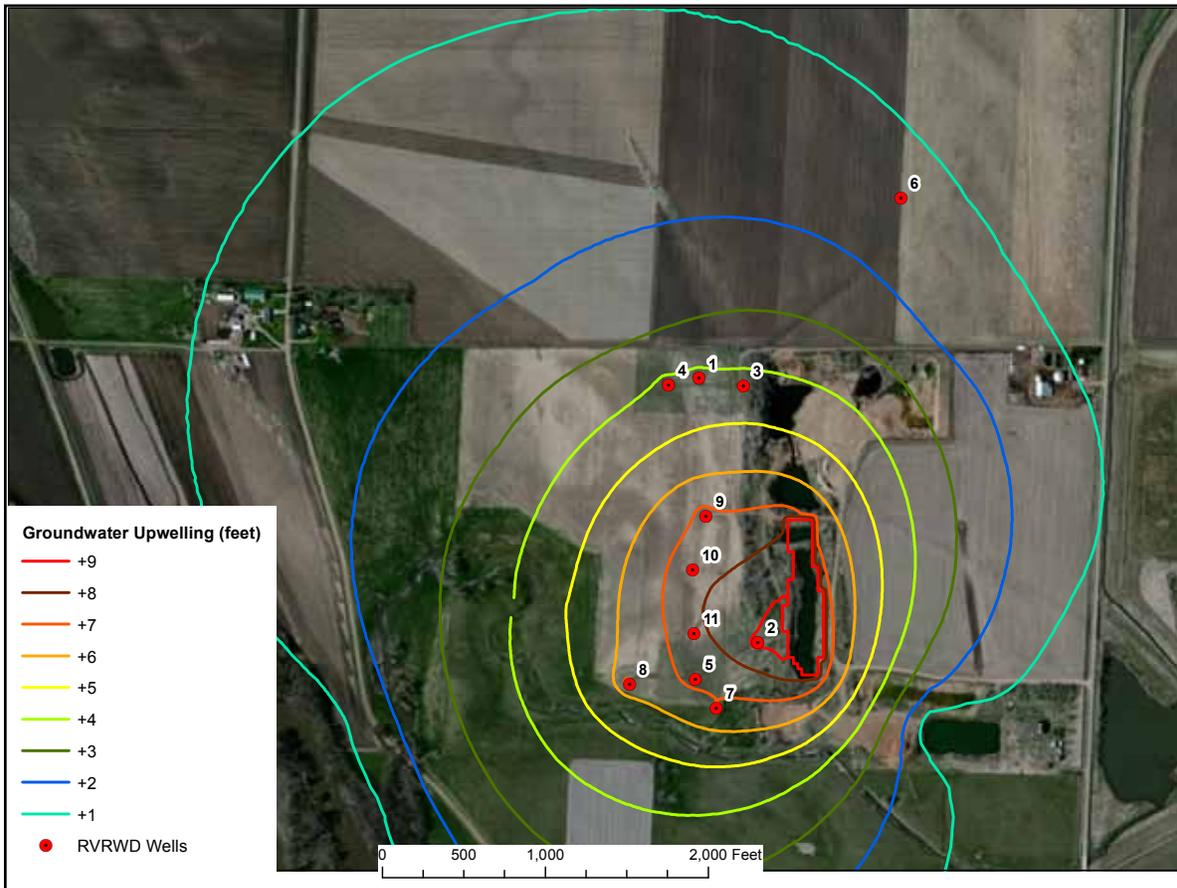
**Figure 12.** Simulated rise (upwelling) in the water table caused by proposed recharge basin.
