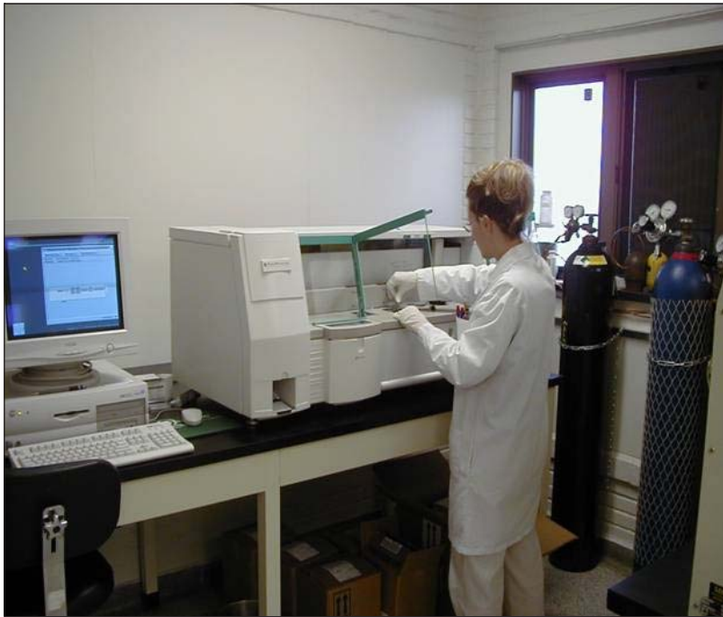
Figure 2. DNA ribotyping is performed at the University of Iowa Hygienic Laboratory using the Riboprinter® Microbial Characterization System.
