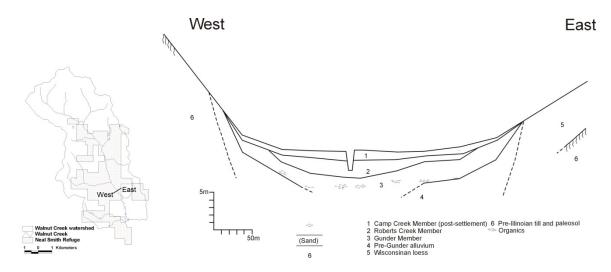
**Figure 2-3:** Cross section across the floodplain of Walnut Creek showing alluvial stratigraphy (modified from Schilling et al., 2004; Schilling et al., 2006).
