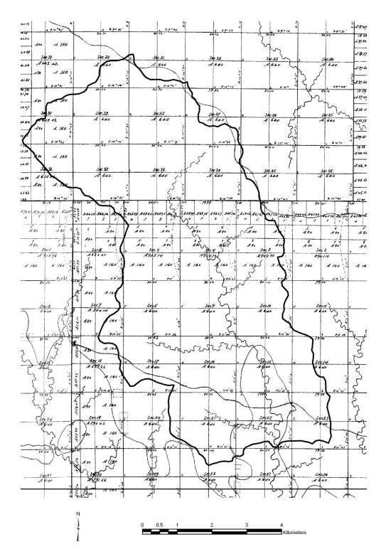
Figure 2-6: Stream channel delineated in 1847 GLO survey.
