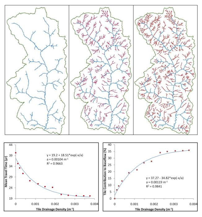
**Figure 3-4:** Hypothesized extent of tile drainage along grass waterways in Walnut Creek watershed (top middle). No drainageway tiling (top left) and maximum tile drainage extent (top right) were included as end members in modeling simulations. Increasing tile drainage density decreases mean travel time (bottom left) and increases tile flow contribution to baseflow (bottom right) (modified from Jindal, 2010 and Schilling et al., 2011).
