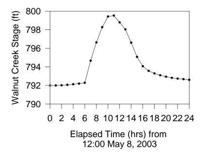
Figure 3-10: Hydrograph of Walnut Creek discharge that shows the flashy nature of streamflow in the incised channel. Discharge increased and decreased nearly eight feet during a 12-hour time period.
