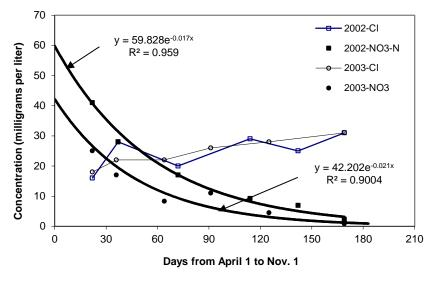
Observed nitrate decay in monitoring well D-4S located in drainageway during 2002 and 2003. Chloride concentrations are shown as a conservation-ion reference (after Schilling et al., 2007)
