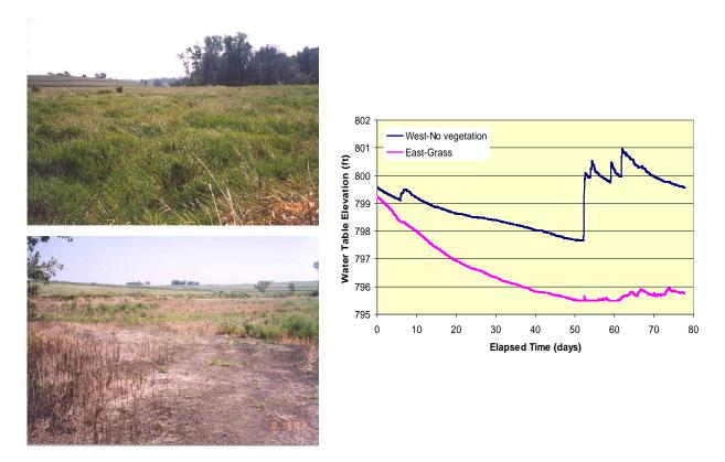
**Figure 3-8:** Water table behavior beneath grass cover on east side of Walnut Creek floodplain compared to groundwater below bare soil on west side during the July 21 to September 11, 2003 (modified from Zhang and Schilling, 2006).
