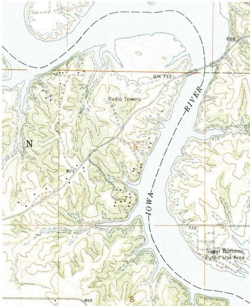
Figure 6. Portion of Ely, Iowa, 7½' topographic quadrangle. The arrangement and spacing of the contour lines (brown) represent the shape and relief of the land surface. This area along the Iowa River-Coralville Reservoir north of Iowa City, shows County Hwy. F28 from North Liberty to Mehaffey Bridge and Stainbrook Geological Preserve. Scale is 1:24,000 or 1 inch = nearly .4 mile. Compare with figure 7.
