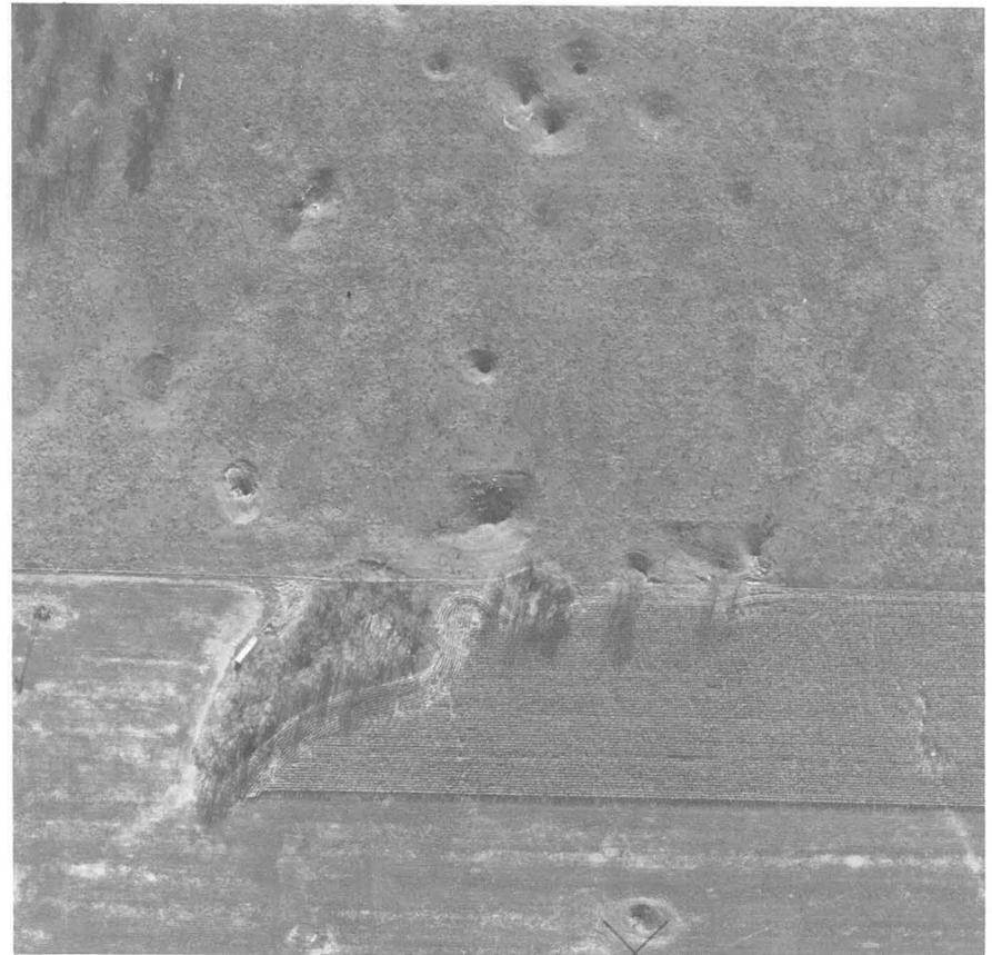
Figure 66. This vertical view of farm fields along Rt. 218 north of Floyd in Floyd County shows numerous circular depressions of sinkholes, characteristic features of karst topography. Solution of underlying limestone resulted in collapse of the land surface. These areas, unusable for crop production, may contain isolated stands of timber, ponded water, or glacial erratics moved out of nearby fields. Photo by Paul G. Allee and Stanley C. Grant.
