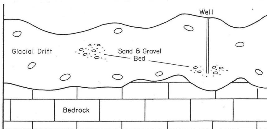
A glacial-drift aquifer is composed of thin, discontinuous sand and gravel zones within less permeable drift materials.
