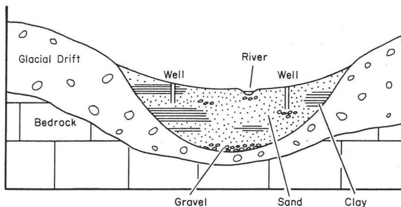
Alluvial aquifers are sand and gravel deposits close to the surface, along major stream valleys.
