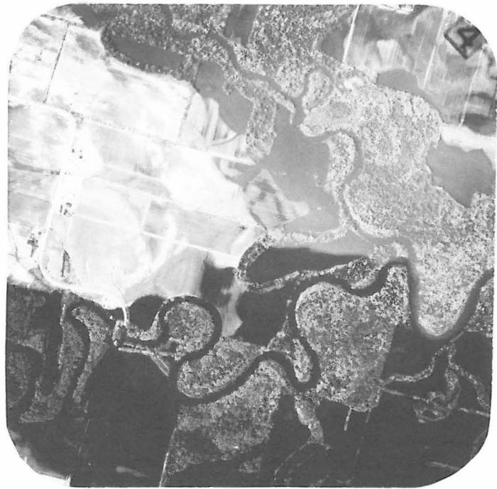
Plate 1. Comparison of red, A (595–685 nm) and infrared, B (740–900 nm) bands imaging April, 1973 flood shortly after the flood crest. The junction of the North and South Skunk Rivers represent two streams with unlike sediment load at the time these images were produced. Notice that the contrast between the soils and water is greater in the infrared band for both the high sediment load stream (North Skunk) and the low sediment load stream (South Skunk).
