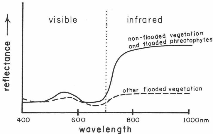
Figure 5. Relative Reflectance of Vegetation after Flood Recession.
