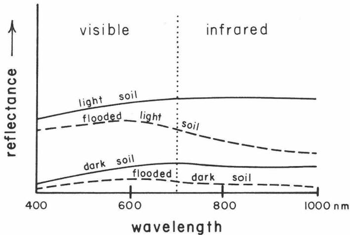
Figure 4. Relative Reflectance of Soil after Flood Recession.
