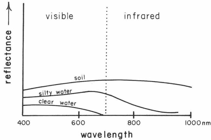
Figure 3. Relative Reflectance of Water and Sand at Flood Crest.
