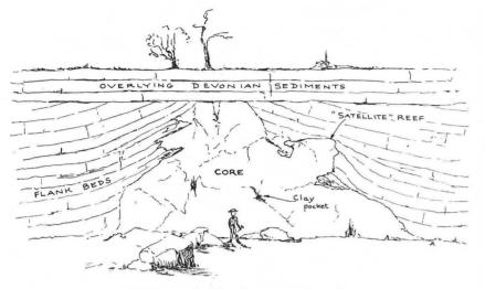
FIGURE 4. Sketch of a Typical Bioherm
