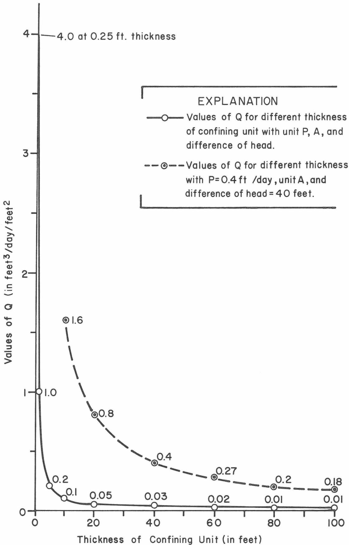
**FIGURE 2.** Values of Q for different thicknesses of P and A.
