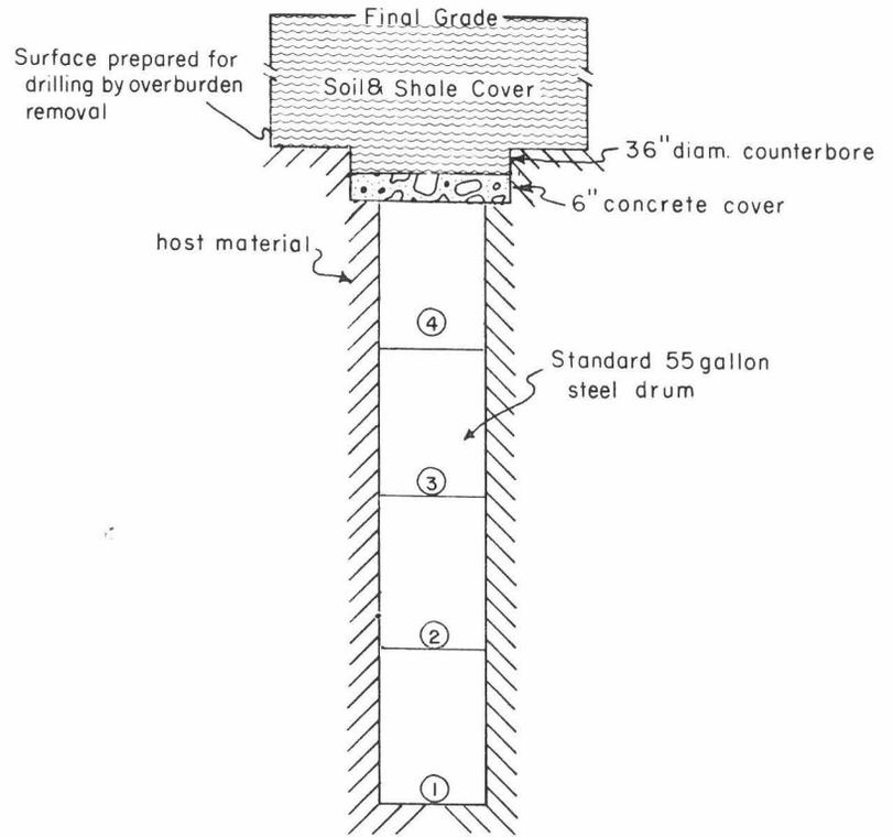
Vertical Section of a Bored Storage Shaft
