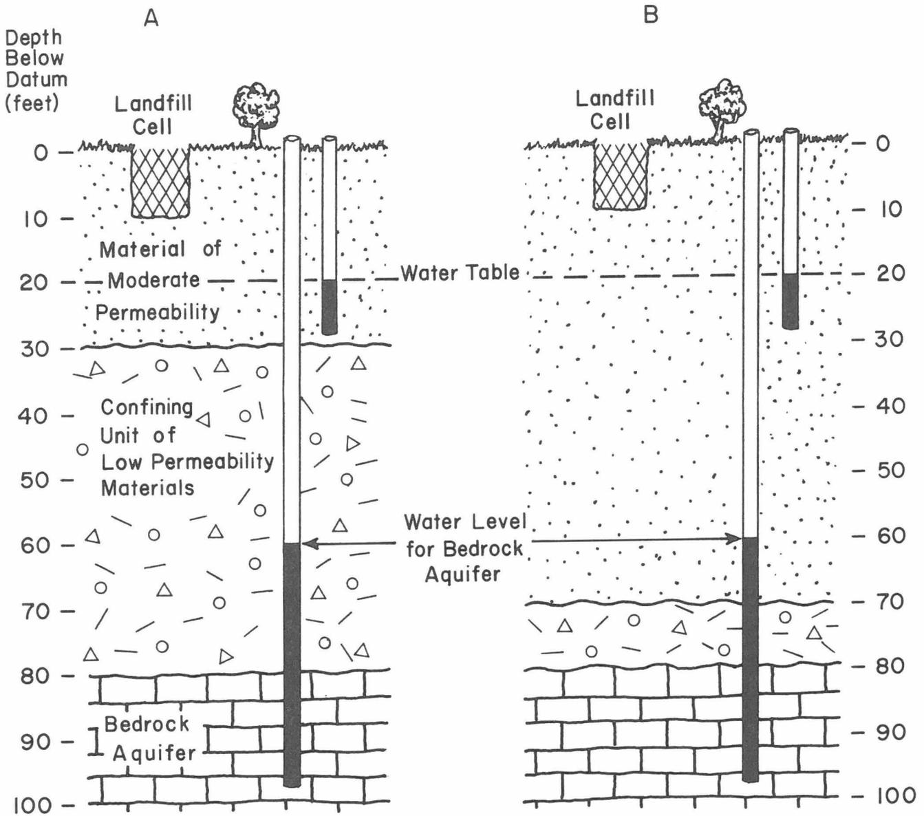
**FIGURE 3.** Cross-sectional diagrams showing the effect of different thicknesses of confining unit.
