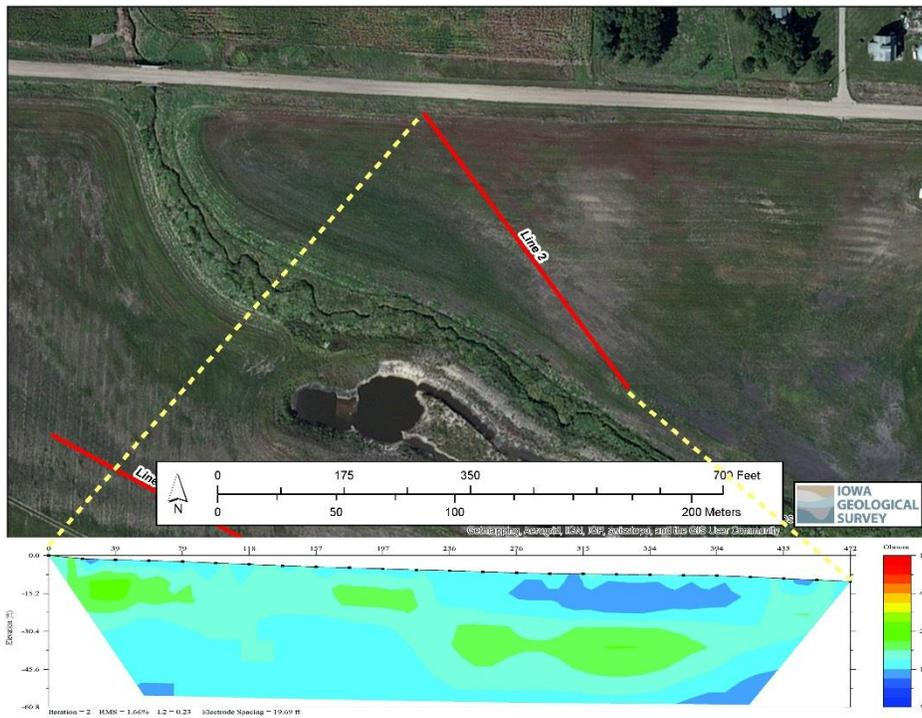
2) Electrical resistivity transect along Line 2 running north of the recharge basin.
