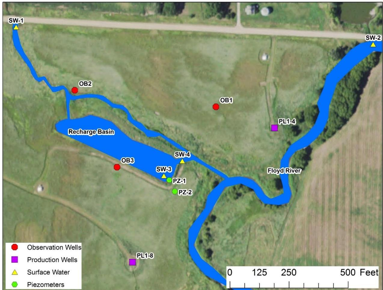
**Figure 4.** Water monitoring at RWS#1 consisting of four surface water locations (SW-1, SW-2, SW-3, SW-4), three groundwater observation wells (OB1, OB2, OB3), and two piezometers in the recharge basin sediments (PZ-1, PZ-2).
