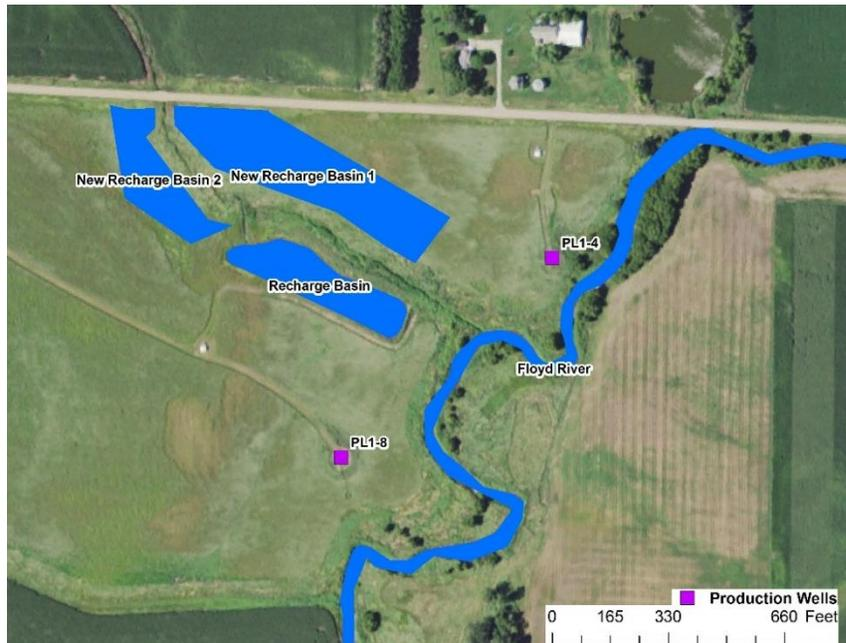
**Figure 14.** Location of two proposed new recharge basins.
