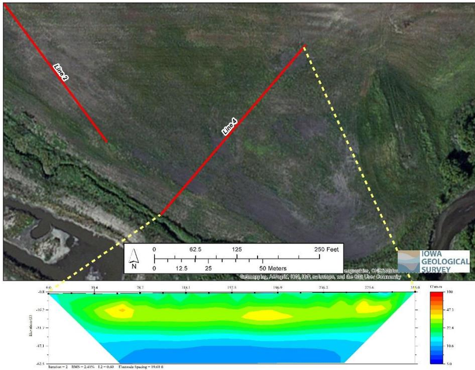
4) Electrical resistivity transect along Line 4 running north of the recharge basin.
