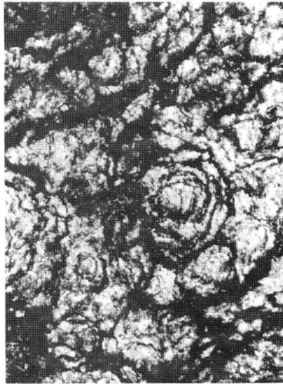
D. Thin section parallel to bedding; notice the fibrous carbonate bundles and the clay concentration surrounding the bundles.
