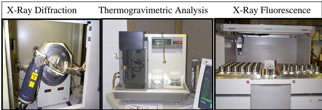
Figure 4. Chemical testing instruments.
