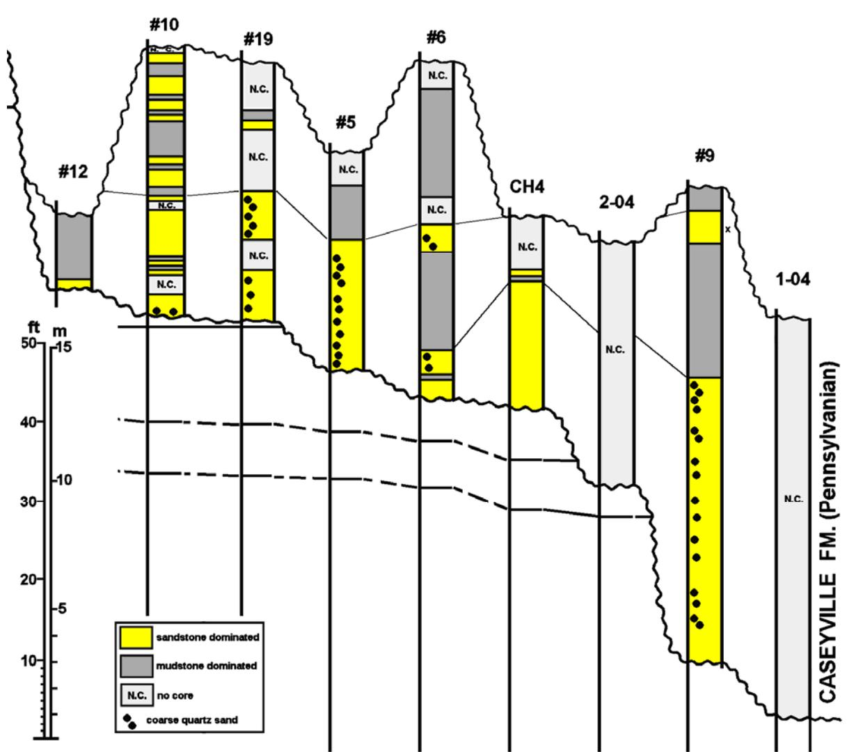
**Figure 17.** Geologic cross section of the Pennsylvanian of Klein Quarry constructed from cores drilled at the quarry. Core #5 was sampled by Brian Witzke for miospores at 27 feet and Core #6 at 50.7 feet. A listing of the resulting taxa can be found in Appendix A. Some of the more significant taxa are illustrated in Plate 1. Note incision into underlying Devonian limestone.
