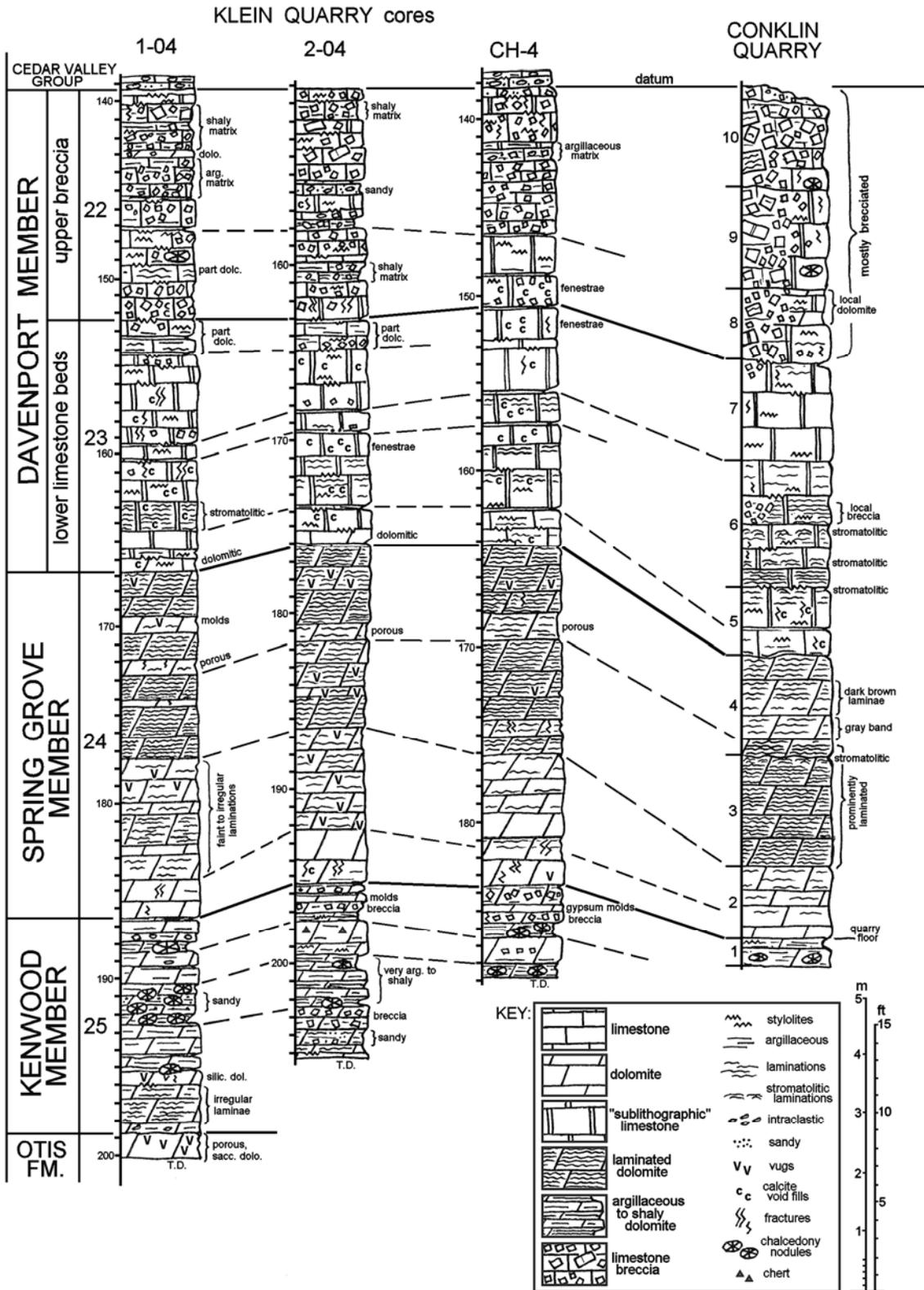
**Figure 2.** Graphic stratigraphic sections and correlation of Wapsipinicon Group at the Klein and Conklin quarries. Unit numbers for Conklin section from Witzke, Bunker, and Glenister (1999).
