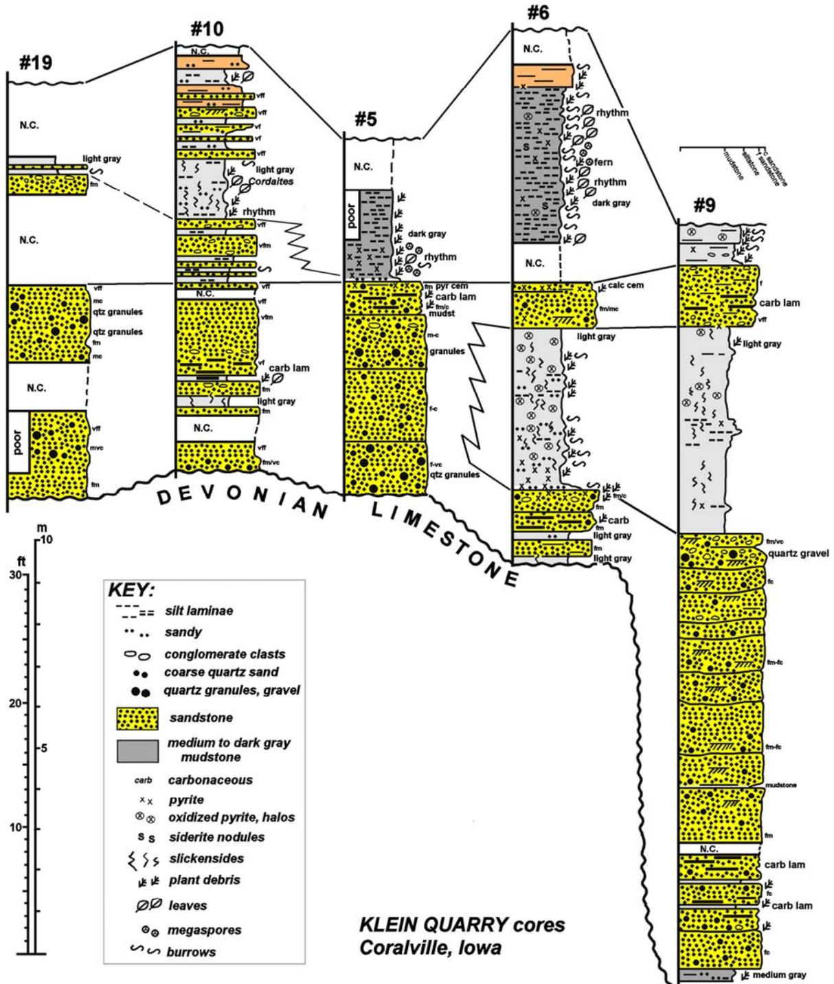
**Figure 18.** Close up, more detailed view of the geologic cross section in Figure 17. Core #5 was sampled by Brian Witzke for miospores at 27 feet and Core #6 at 50.7 feet. A listing of the resulting taxa can be found in Appendix A. Some are illustrated in Plate 1. Note presence of rhythmites in mudstone and incisement into underlying Devonian limestone.
