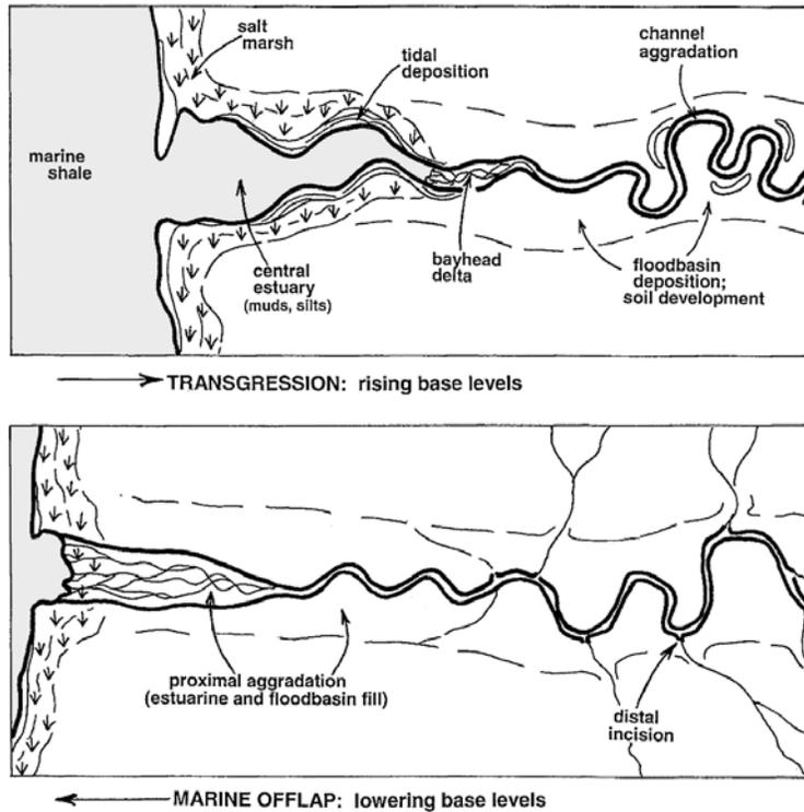
**Figure 15.** Lower Pennsylvanian estuaries in southeast Iowa during sea level rise (top) and during sea level fall (bottom), note upstream channel aggradation and tidal deposition in top diagram and channel incisement in bottom diagram. Estuaries may have reached over 400 km into Johnson County as evidenced by tidal rhythmites in Klein Quarry (Witzke, 2010).
