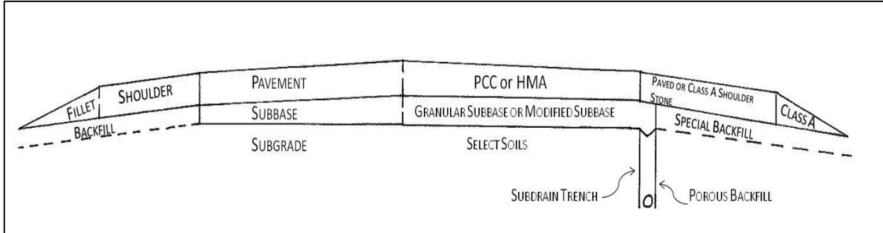
Figure 3. Highway Cross-section.
