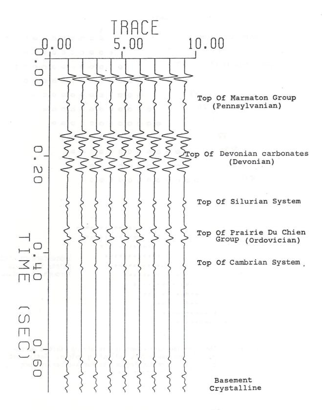
Figure 4. Synthetic seismogram for Malvern model.
