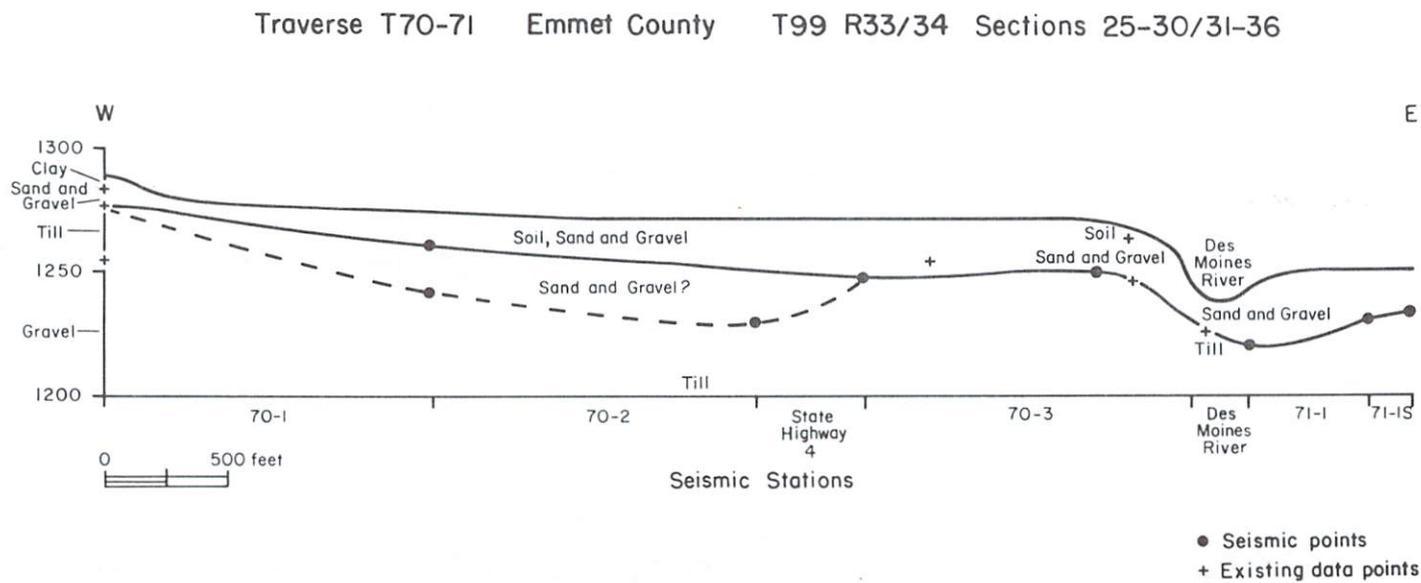
Figure 29. Seismic profile section: T70-71.
