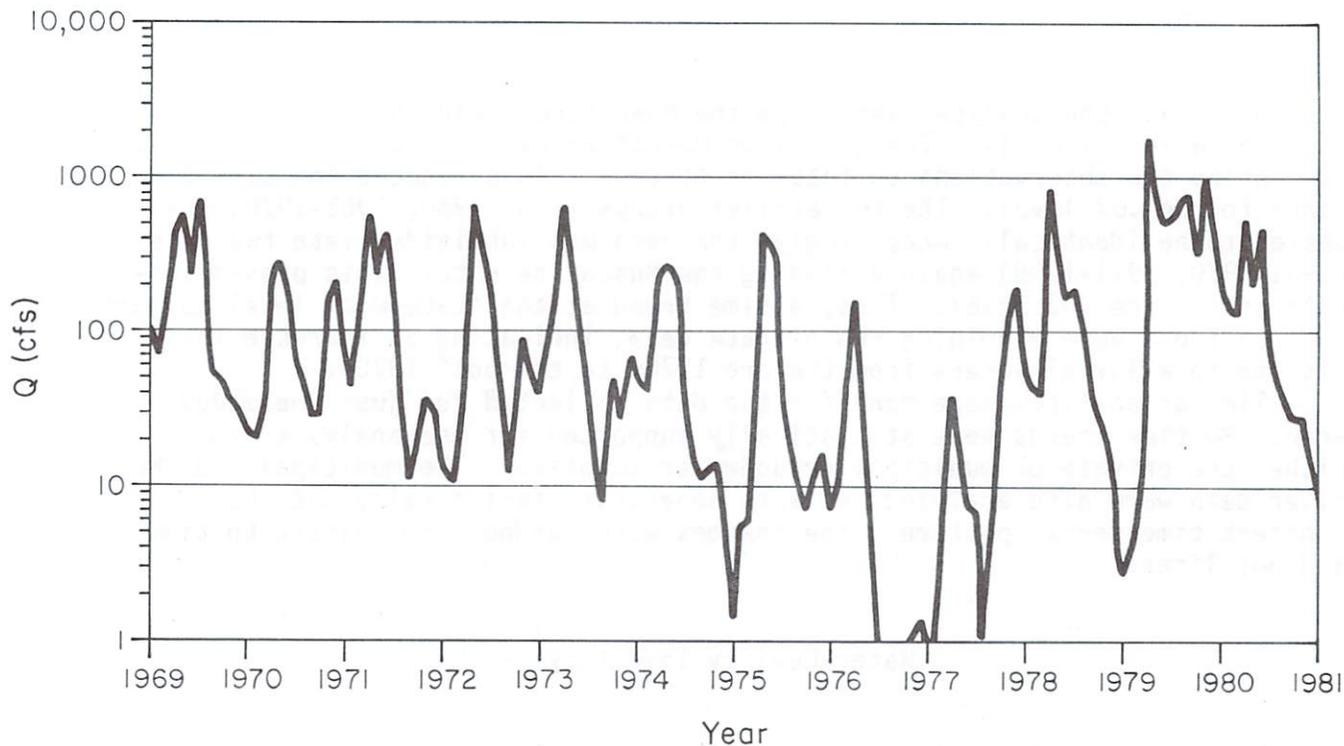
Figure 56a. Monthly minimum discharge data from Estherville (Emmet Co.) gaging station.
