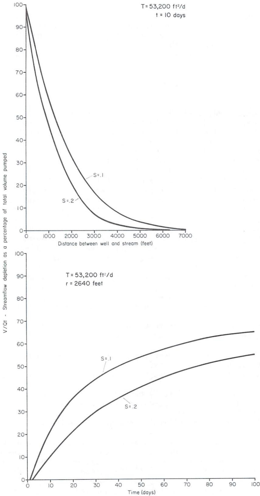
Figure 55. Stream depletion curves showing the effects of time of pumping and distance between the river and the pumped well.
