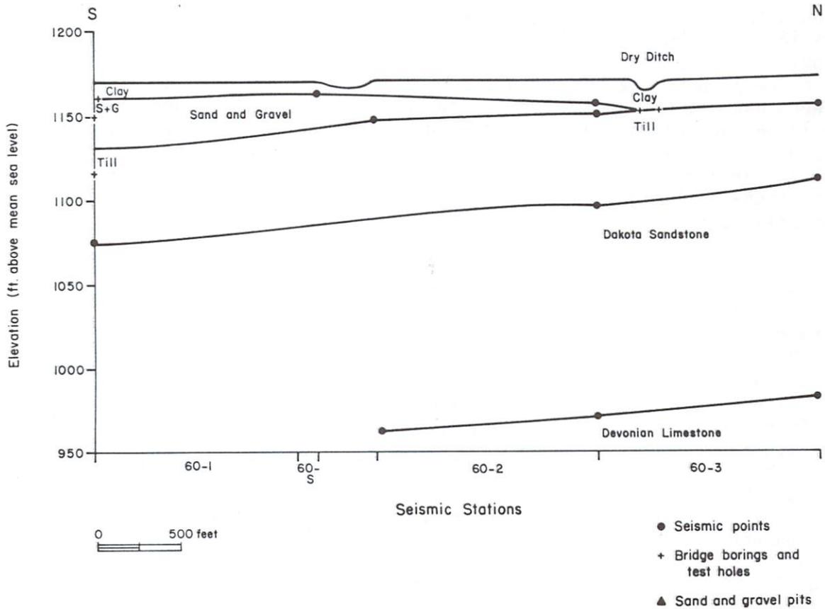
Figure 23. Seismic profile section: T60.
