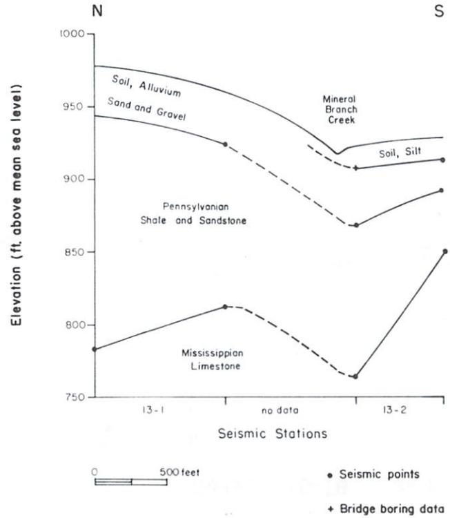
Figure 15. Seismic profile section: T13.
