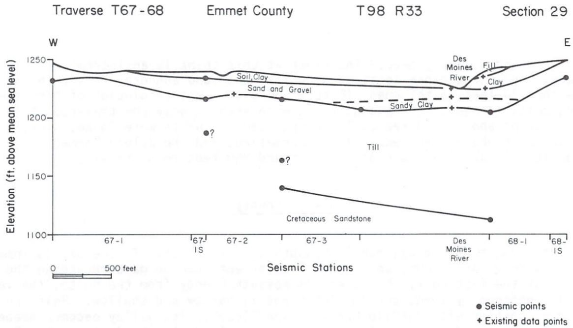
Figure 30. Seismic profile section: T67-68.
