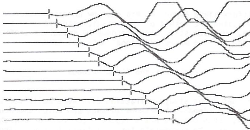
Figure 8. Typical seismogram. Tic marks indicate time of arrival of wave on each channel.
