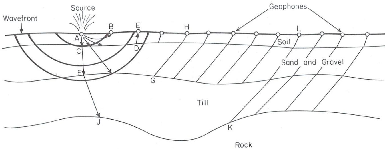
Figure 7. Schematic of sound wave propagation through a typical alluvial sequence. Letters refer to discussion in text.
