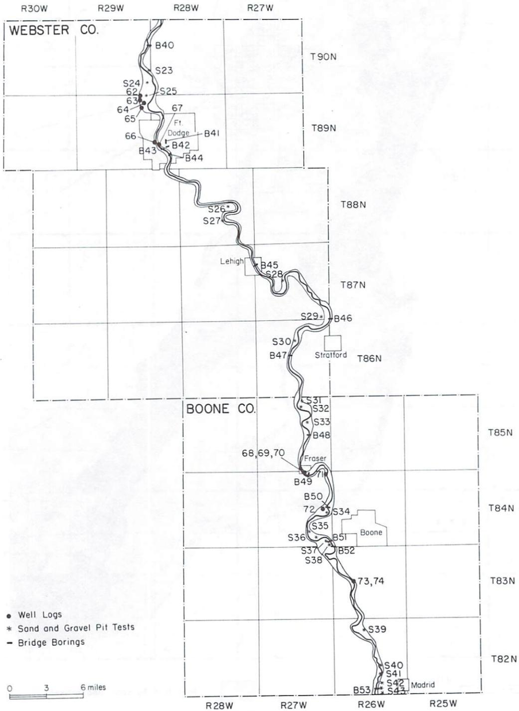
Figure 5. Locations of well log, bridge borings, and sand and gravel pit data: Lower River.
