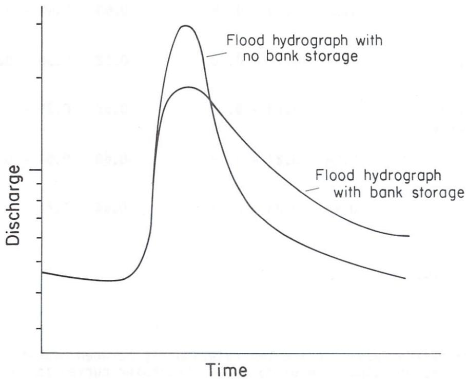
Figure 43. Idealized hydrograph showing the effects of bank storage.
