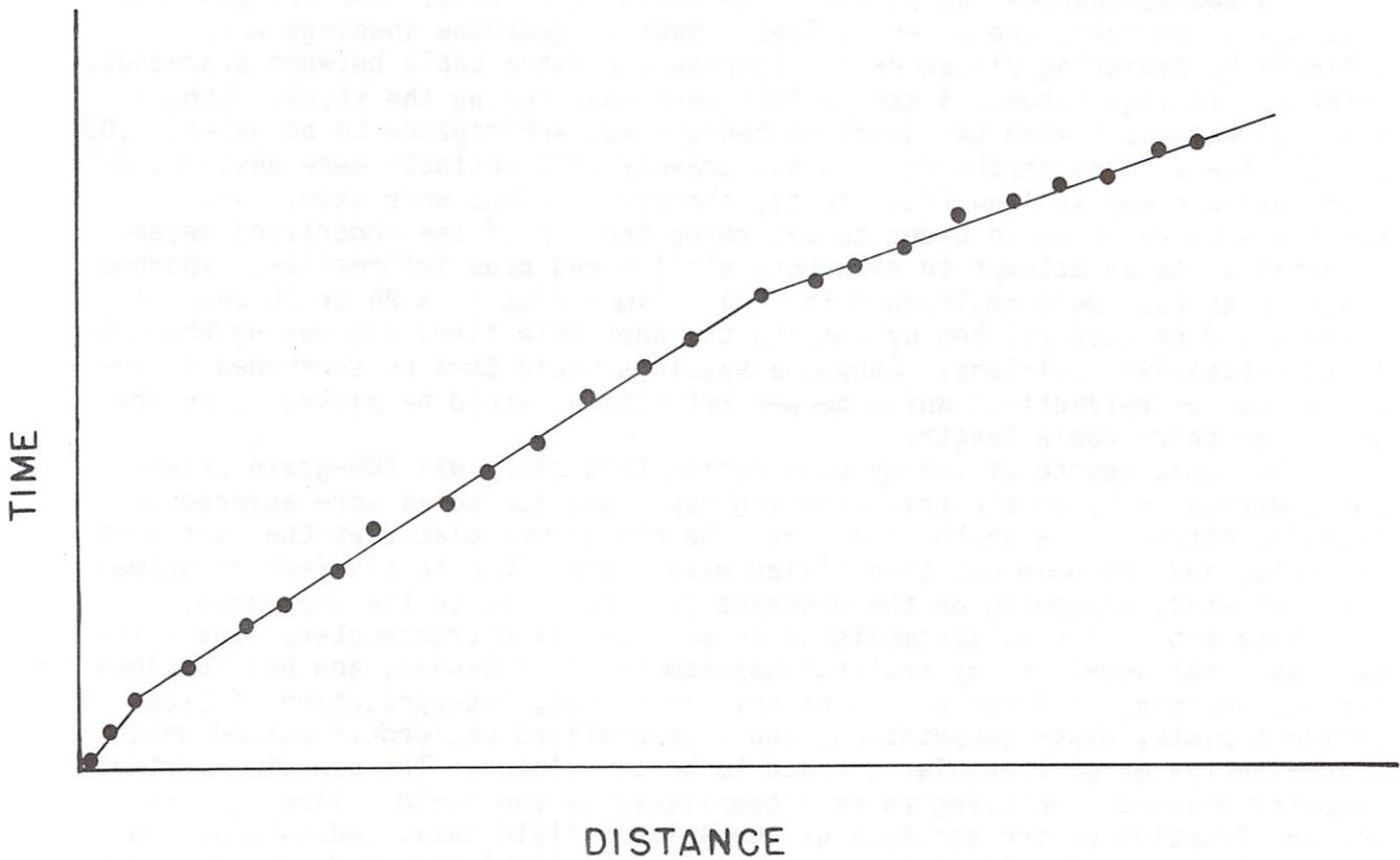
Figure 9. Idealized time-distance graph. Each slope segment represents refractions from a particular interface. The velocity of the unit is equal to the inverse of the slope.
