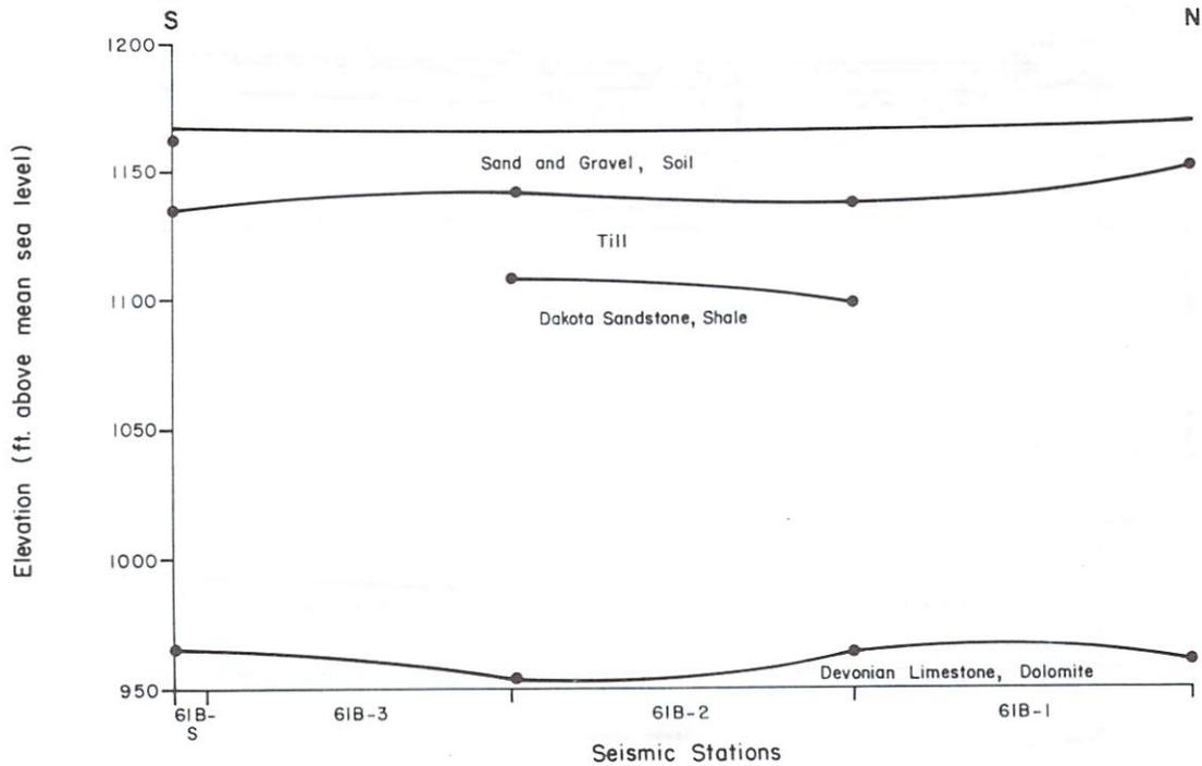
Figure 25. Seismic profile section: T61B.
