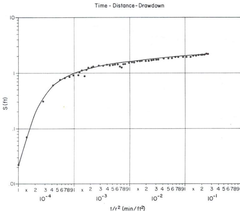
Figure 53. Time-distance drawdown curve.
