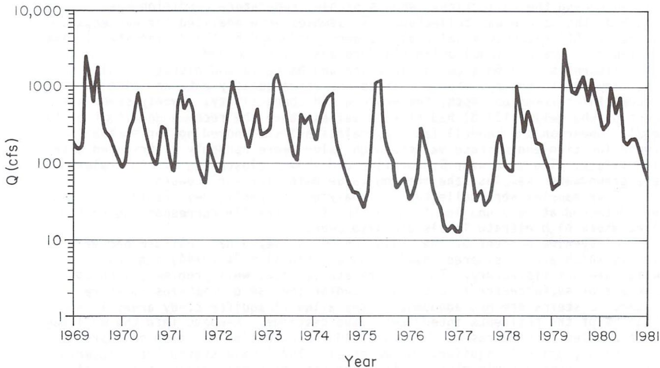
Figure 56b. Monthly minimum discharge data from Humboldt (Humboldt Co.) gaging station.
