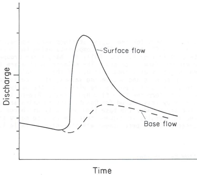
Figure 42. Idealized hydrograph illustrating the relative relationships of surface runoff and groundwater flow.
