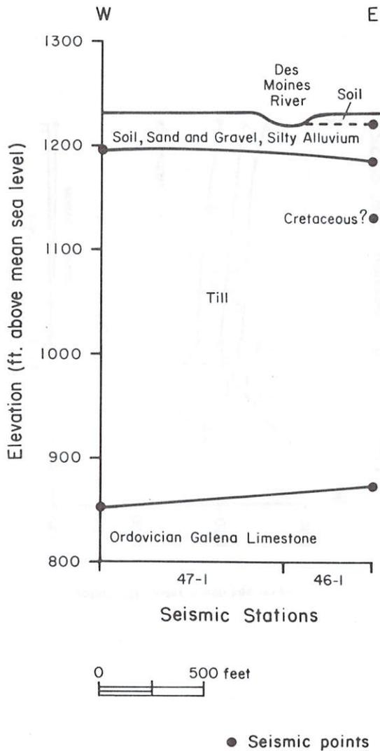
Figure 32. Seismic profile section: T47-46.
