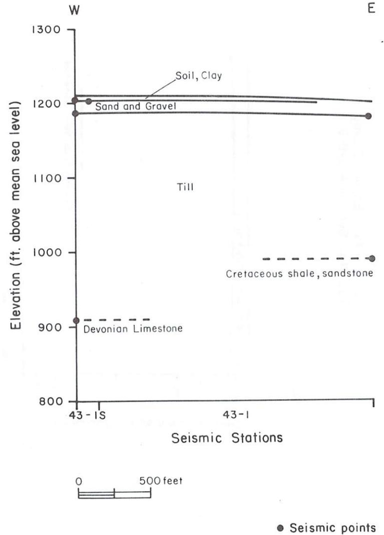
Figure 33. Seismic profile section: T43.
