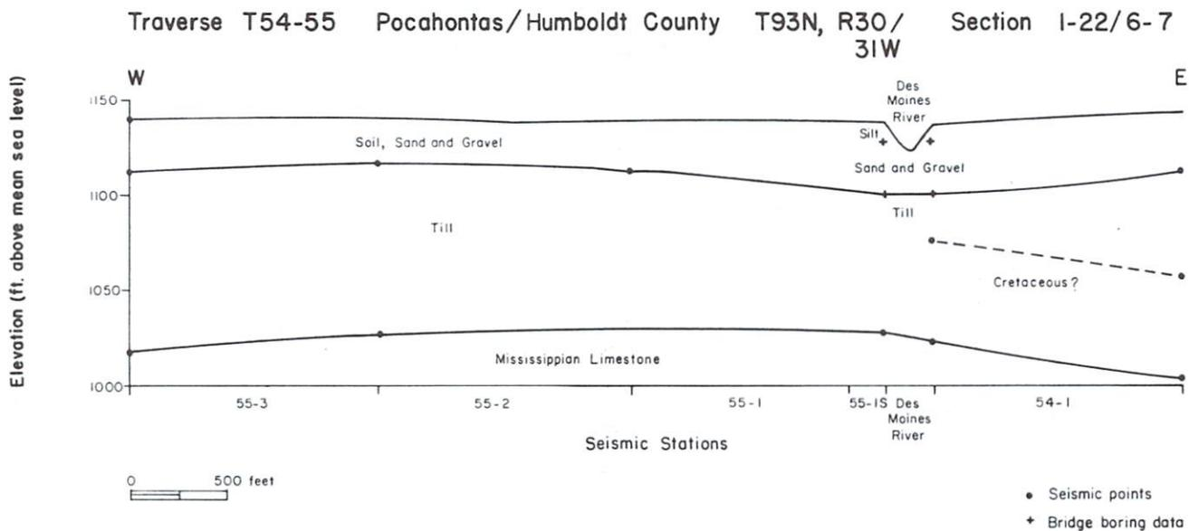
Figure 21. Seismic profile section: T54-55.
