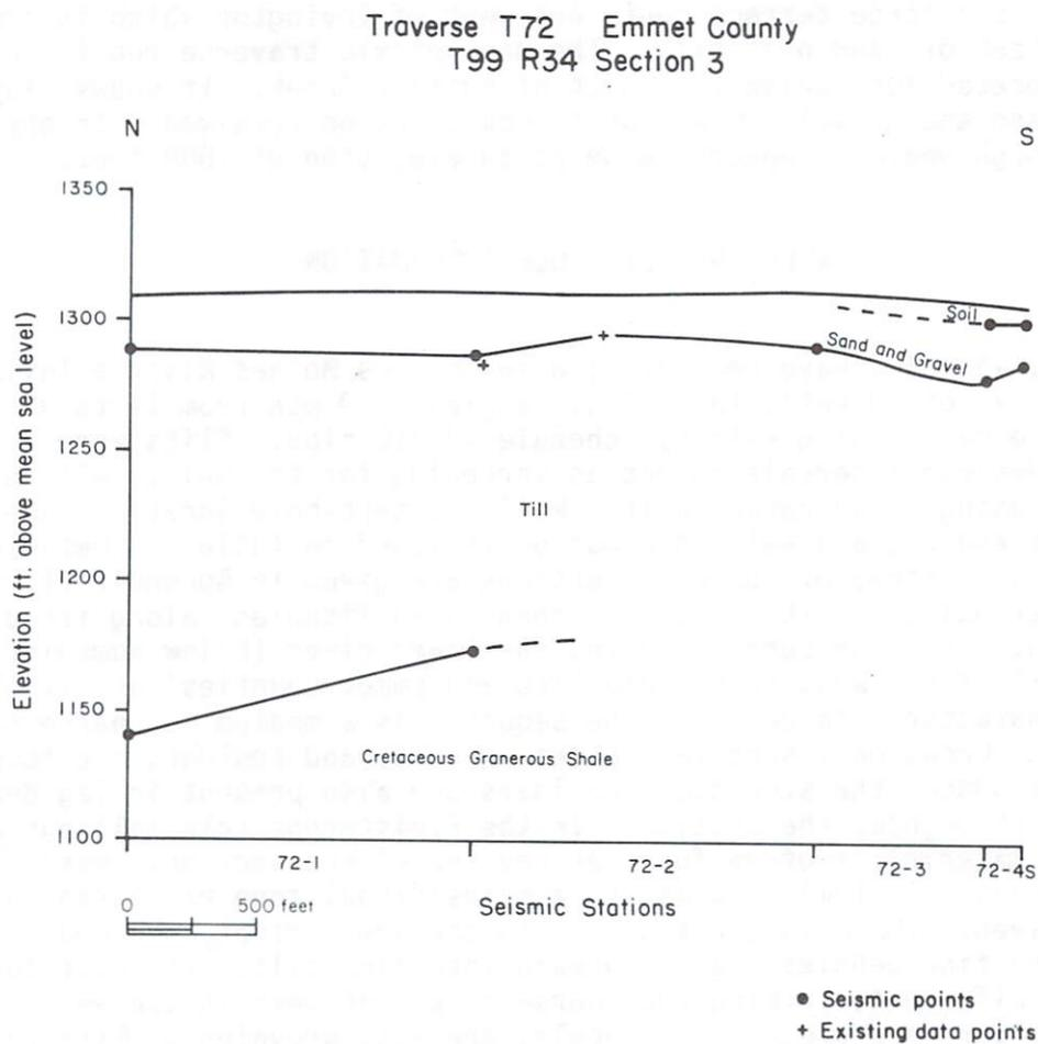
Figure 31. Seismic profile section: T72.
