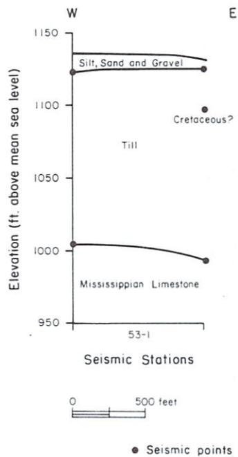
Figure 20. Seismic profile section: T53.
