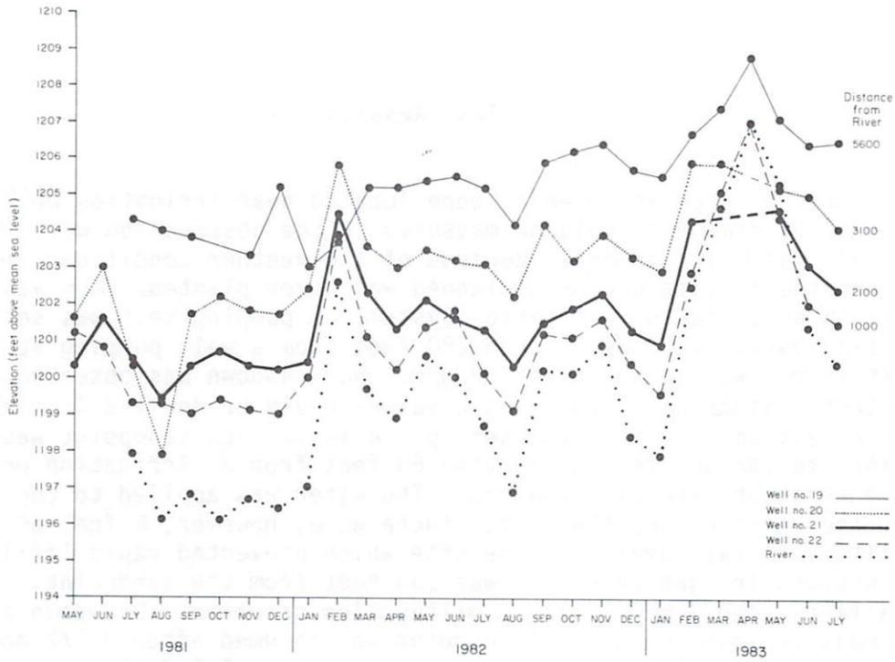
Figure 51. Static water levels with time in a selected set of wells.
