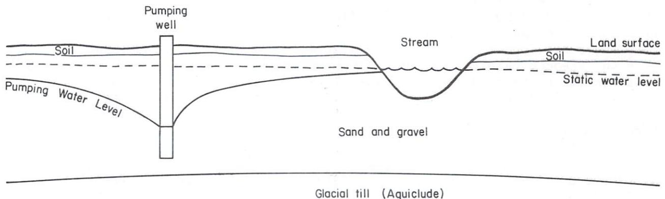
Figure 46. Schematic showing relationship between static and pumping water levels.
