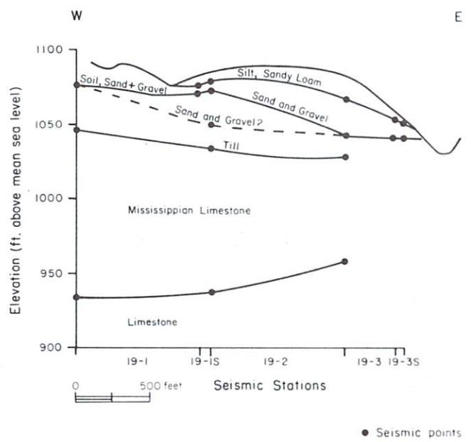
Figure 16. Seismic profile section: T19.
