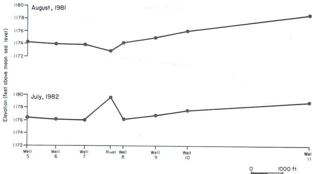
Figure 52. Static water levels at a given time for a selected set of wells.
