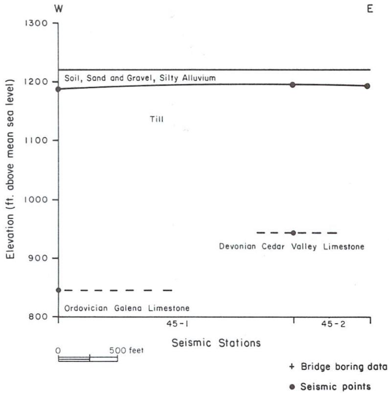
Figure 34. Seismic profile section: T45.
