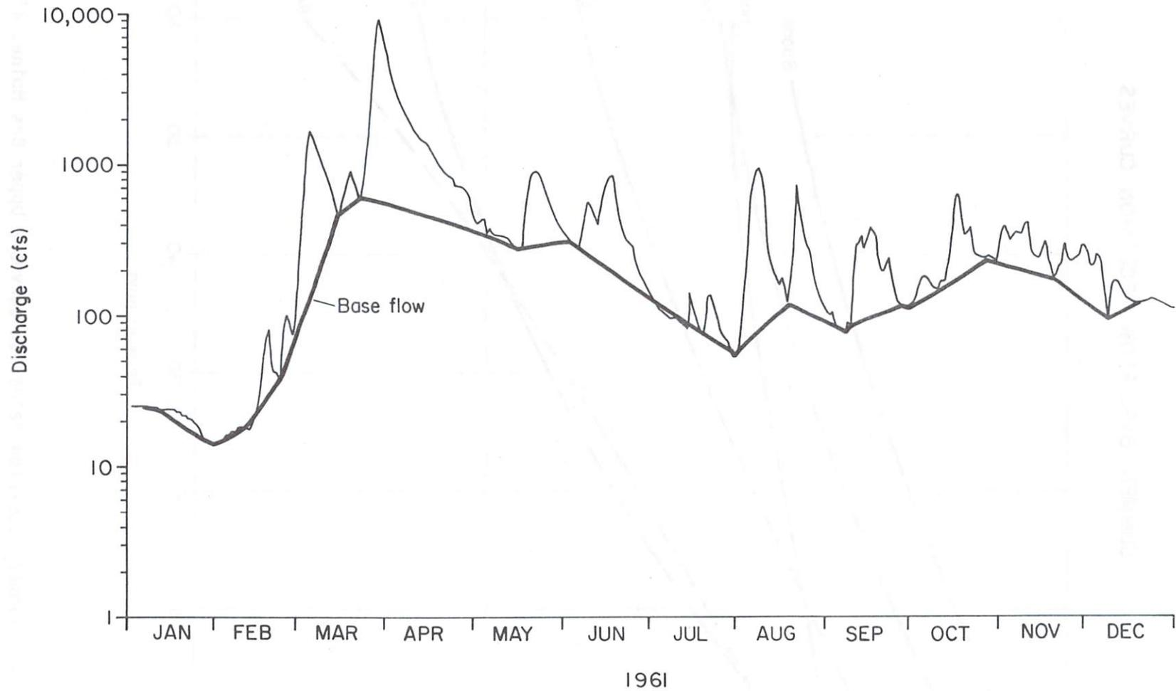
Figure 44. Dakota City hydrograph showing baseflow separation by the method discussed in the report.
