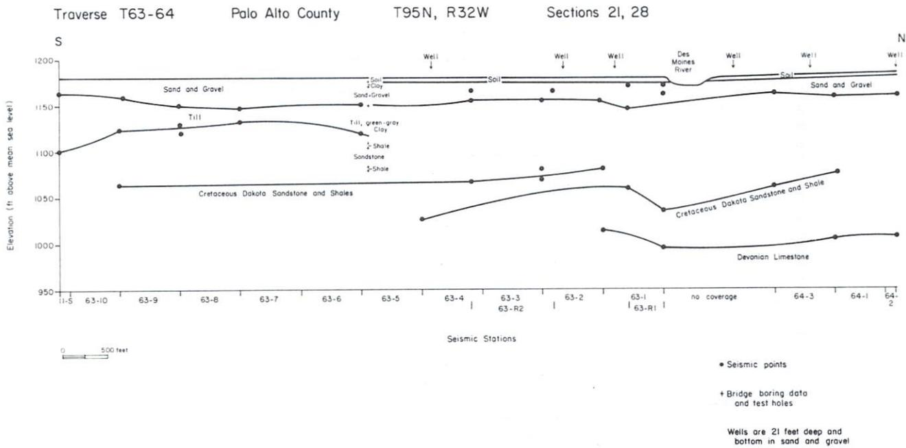
Figure 26. Seismic profile section: T63-64.
