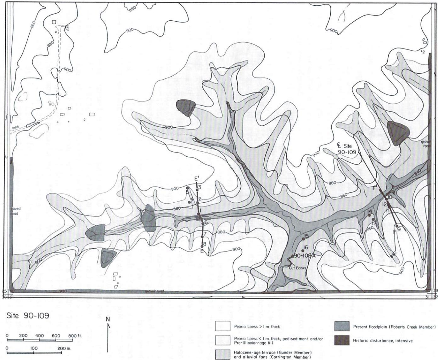
Figure 11. Map of the 90-109 area showing topography, location of borings and cut banks, and generalized distribution of Quaternary materials.
