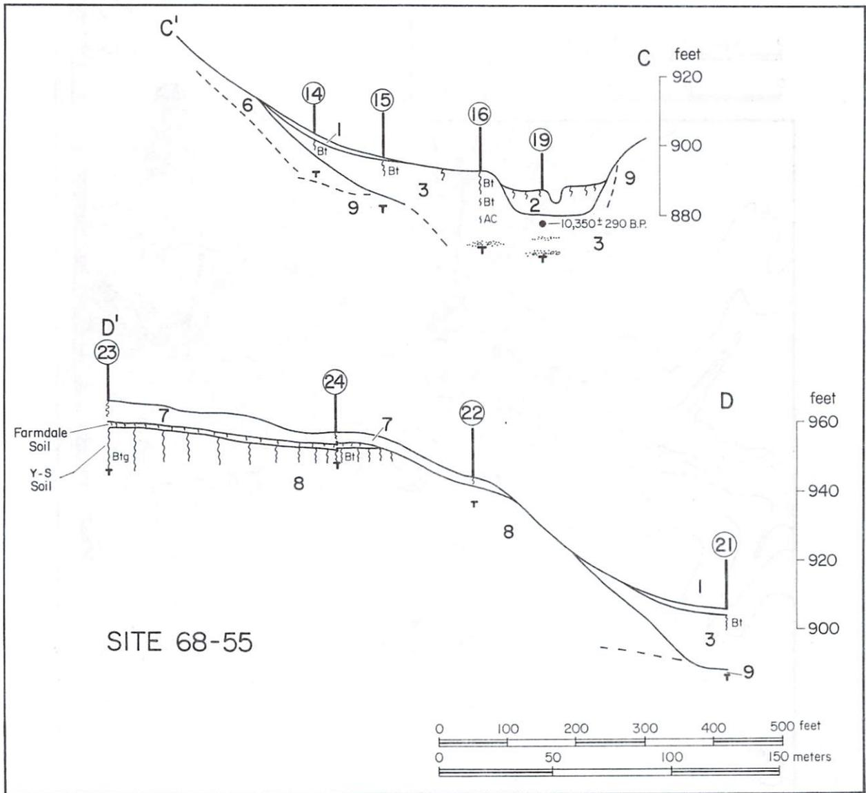
Figure 10. Cross-sections showing stratigraphic relationships among Quaternary materials in the 68-55 area. The location of the cross-sections are shown on Figure 9.
