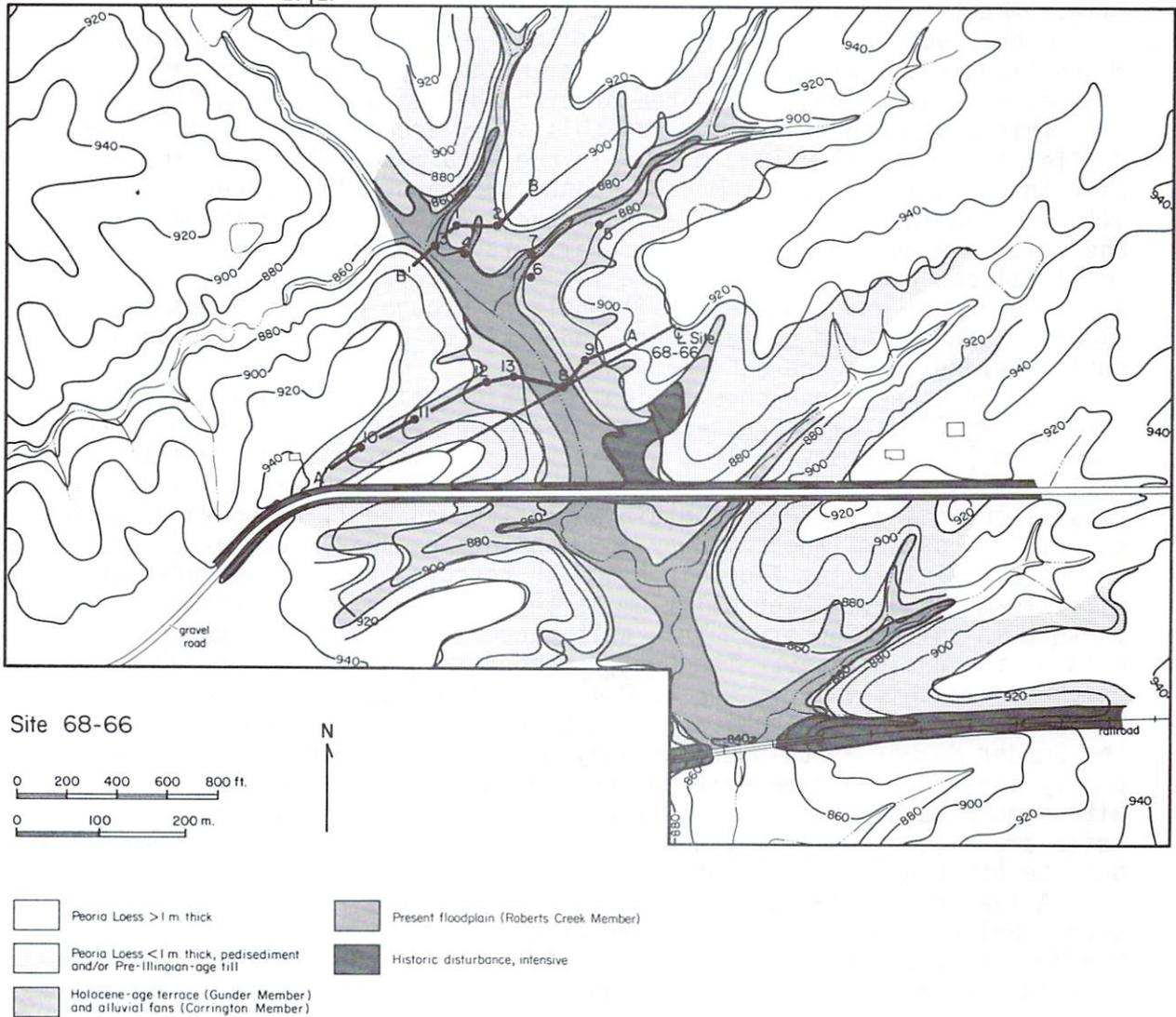
Figure 7. Map of site 68-66 area showing topography, location of borings, and generalized distribution of Quaternary materials.
