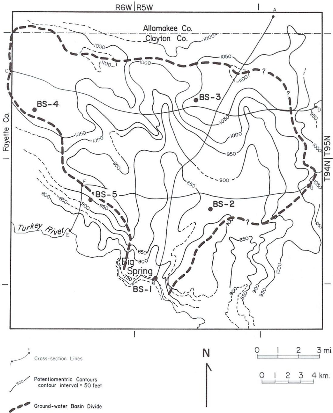
Figure 3. Elevation of the water table/potentiometric surface in the Galena aquifer, and lines of cross-section shown on figures 5 through 7 (adapted from Hallberg et al., 1983).
