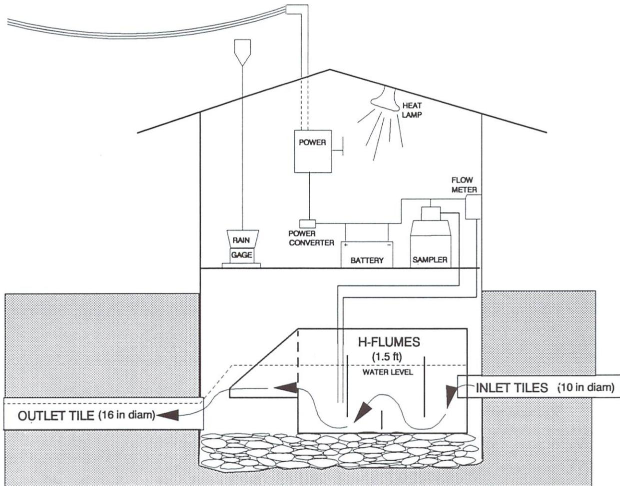
Figure 6. Diagram of Bugenhagen sub-basin instrument shed.
