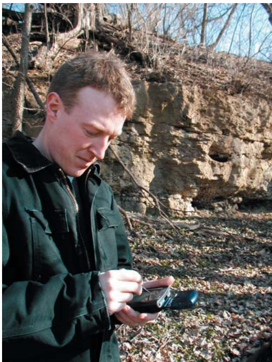
Figure 1. A member of the GIS staff collects data using a Global Positioning System (GPS) receiver. GPS receivers can be modified to collect tabular data on specific characteristics (outcrop, weather conditions, surrounding flora) of the landscape. These data are then downloaded to a computer and tied to the point generated on a GIS file. GPS points provide a more accurate analysis of trends or patterns in natural resources. The ability to enter tabular data at the point of collection ensures accurate attribution and lessens the likelihood of data being mistakenly entered while transferring from a field notebook.
