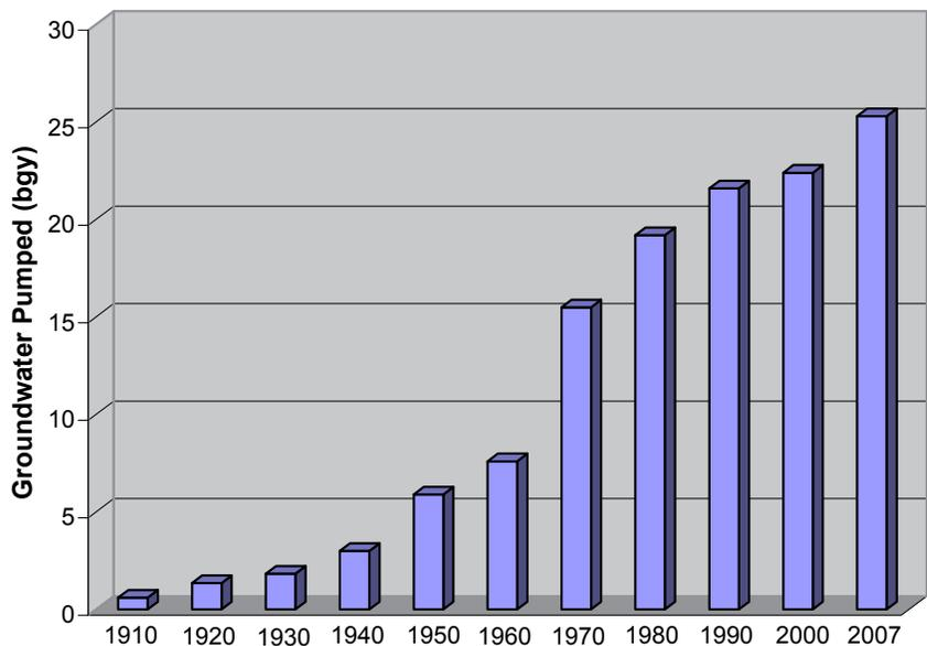
**Figure 2.** Water-use data for the Cambrian-Ordovician aquifer from 1910 to 2007. Data include total yearly volume pumped in billion gallons per year (bgy). Totals include wells completed in more than one aquifer (dual completion wells).
