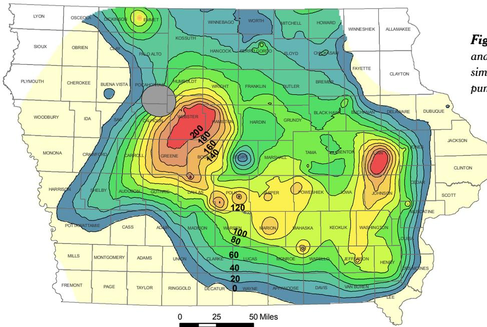
**Figure 4.** Declines in water levels from Horick and Steinhilber (1978) baseline map to computer simulated results in 2029 with a 25% increase in pumping rates.
