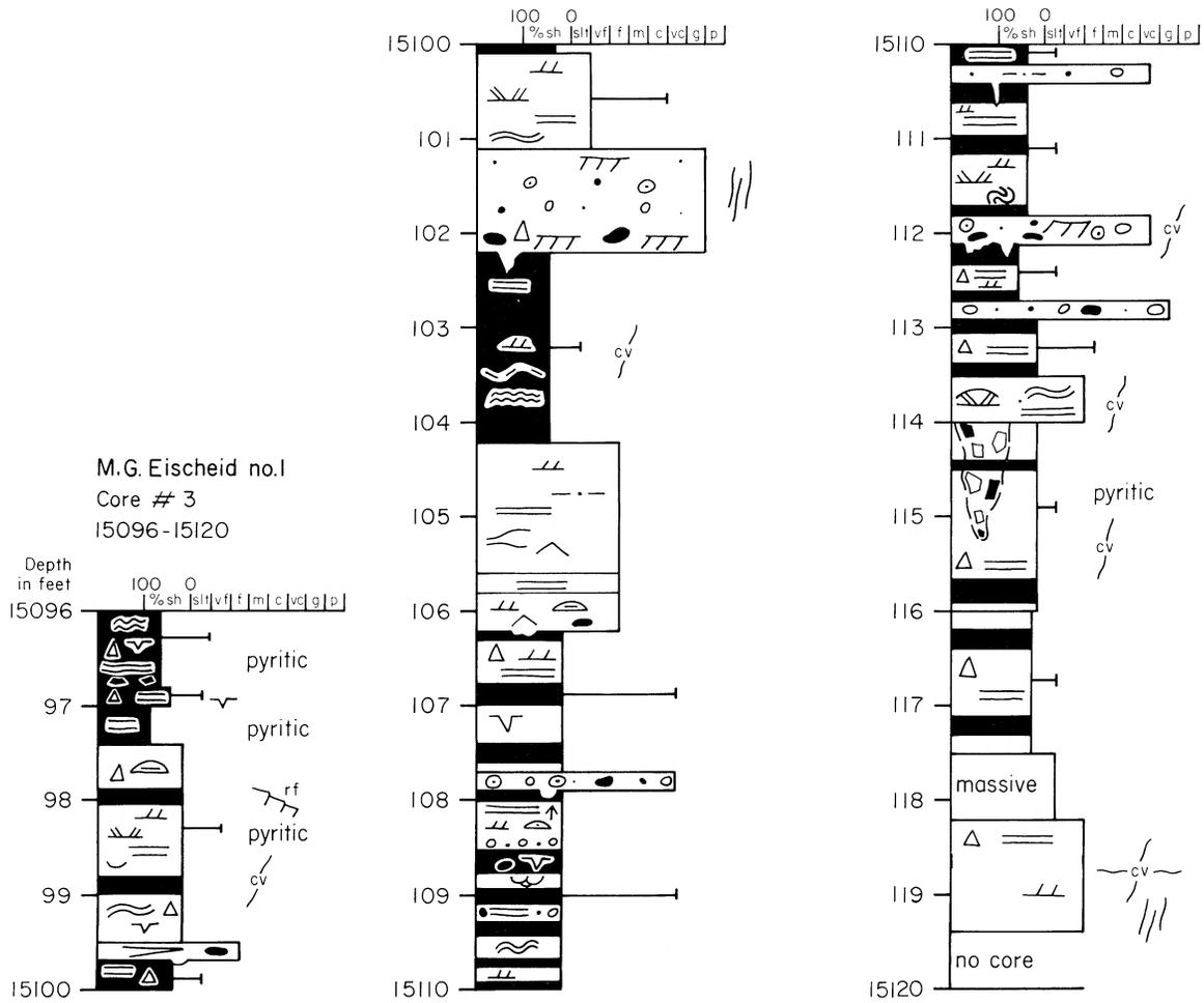
Figure 4. Graphic log of core #3, Eischeid test. Written description in Appendix A.
