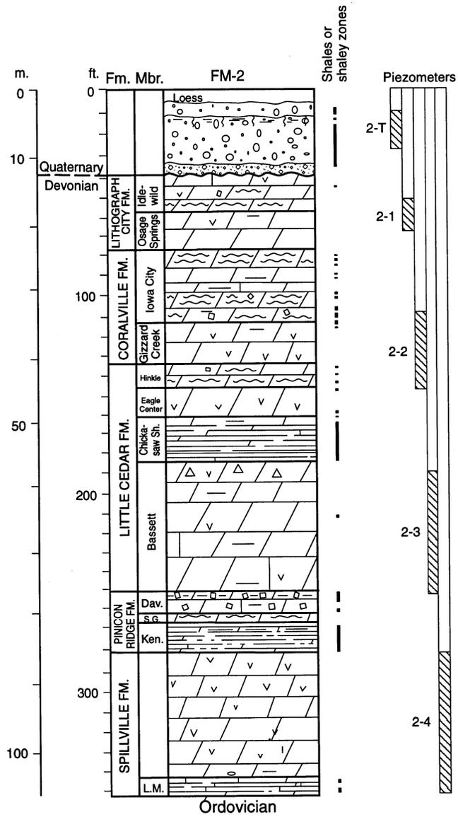
Figure 9. Geologic log, packer-test intervals, and piezometer completions, Site #2.
