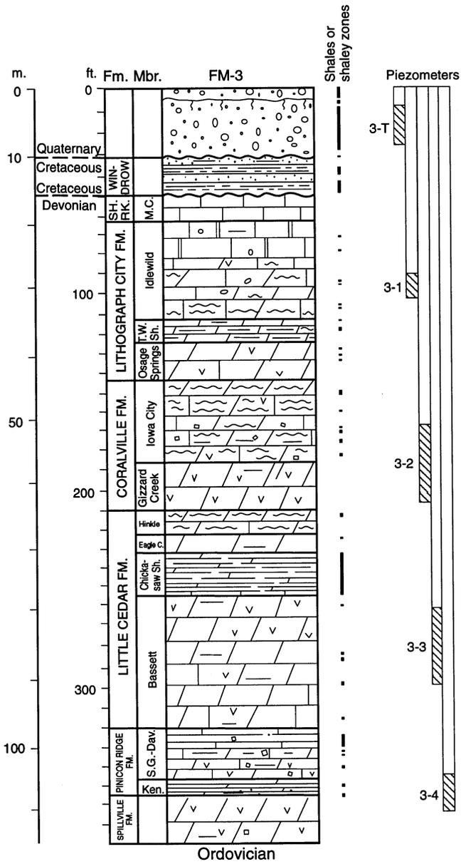
Figure 10. Geologic log, packer-test intervals, and piezometer completions, Site #3.
