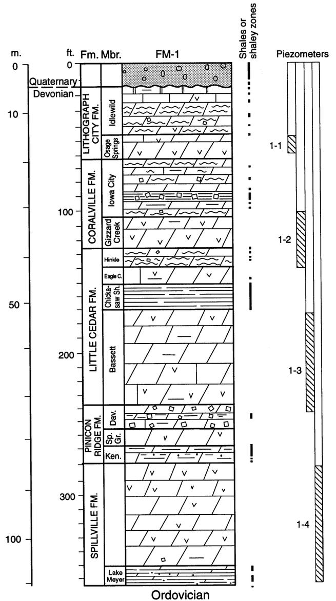
**Figure 8.** Geologic log, packer-test intervals, and piezometer completions, Site #1.
