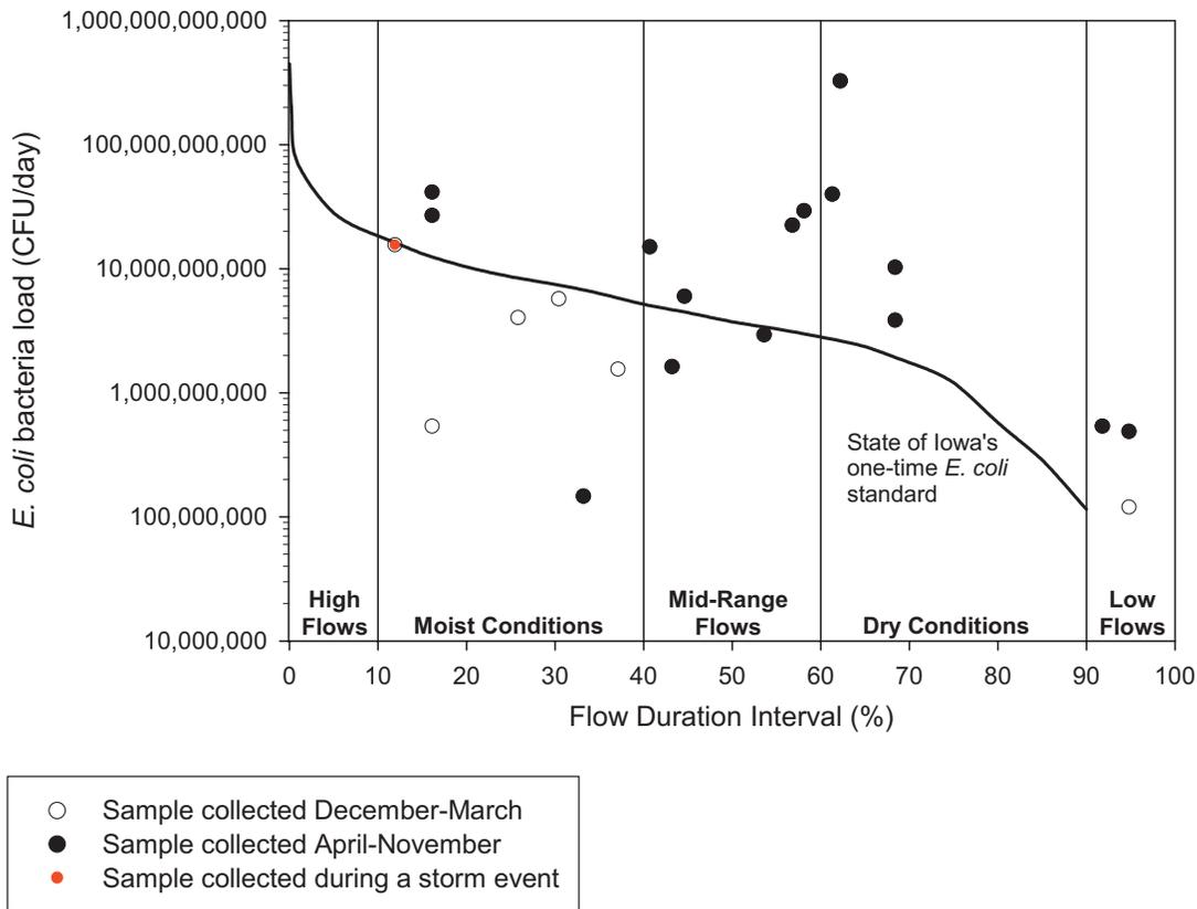
**Figure 6.** *E. coli* load duration curve for Hoover Creek at the gaging station in the Herbert Hoover National Historic Site, 2004 through 2006.
