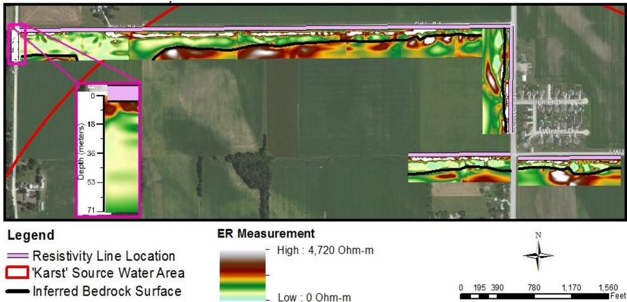
**Figure 4.** Map showing the electrical resistivity depth sections with inferred bedrock surface elevations north of well 9 and 10. Resistivity measurements are shown in Ohm-meters, with higher resistivity in the brown and white color spectrum and lower resistivity in the green and light blue spectrum
