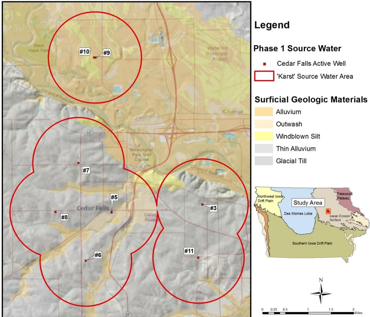
**Figure 3.** Map indicating the surficial geologic materials in the Cedar Falls Source Water Area. The region is dominated by weathered glacial till to the south of the Cedar River, and thick alluvial and eolian (windblown) deposits to the north of the current river channel.
