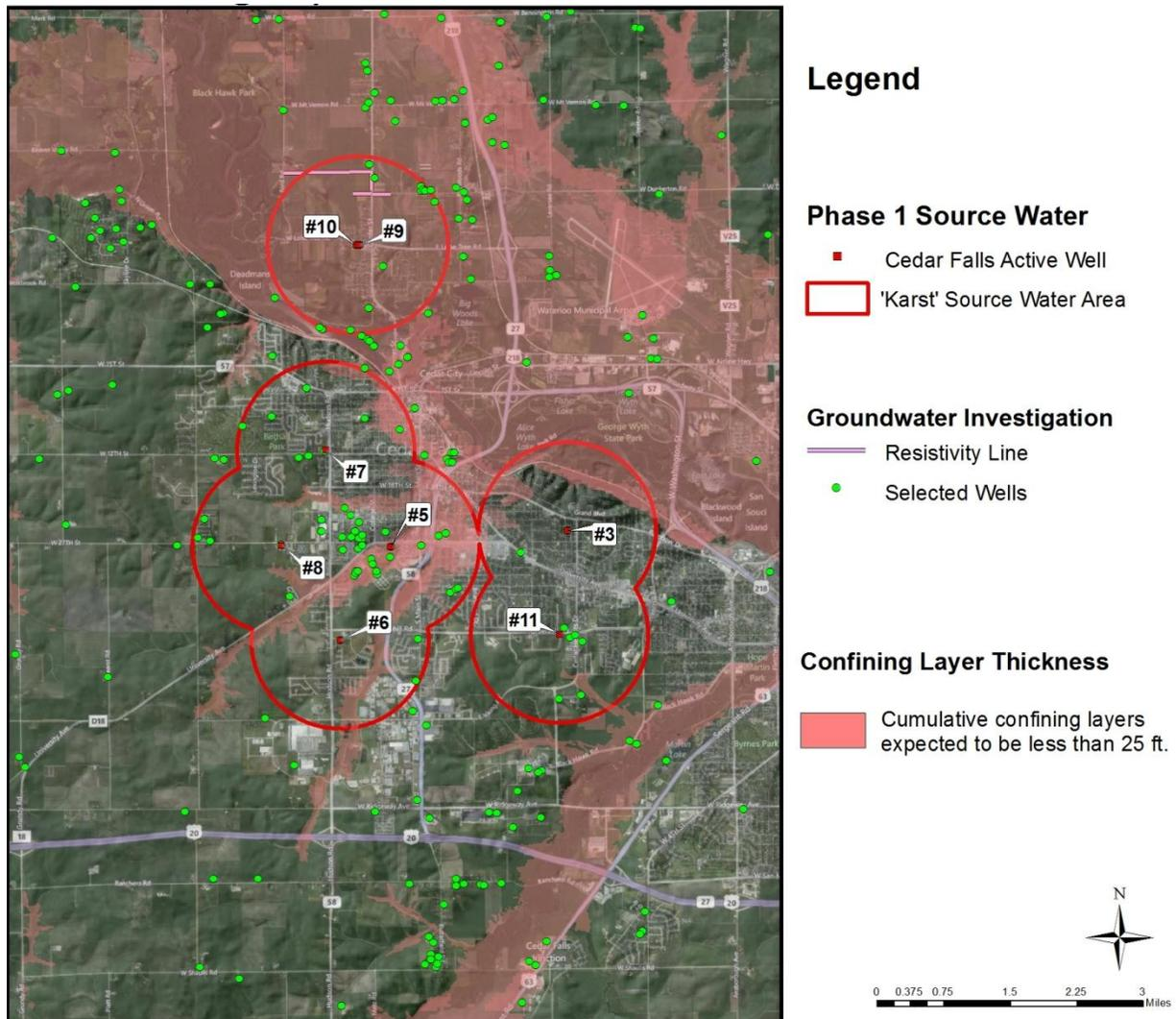
**Figure 6.** Map indicating the estimated confining layer (shale, till, clay) separating the land surface from the Silurian-Devonian bedrock aquifer. Confining layer thickness was estimated using geologic records, soils coverages, and bedrock elevation mapping.
