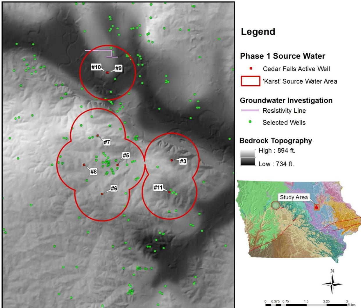
**Figure 5.** Map indicating the bedrock topography, study area, lithologic wells, and geophysical resistivity lines used to determine bedrock topography in the study region. In the study region, the surface unit of bedrock is the Cedar Valley Formation of the Devonian System.
