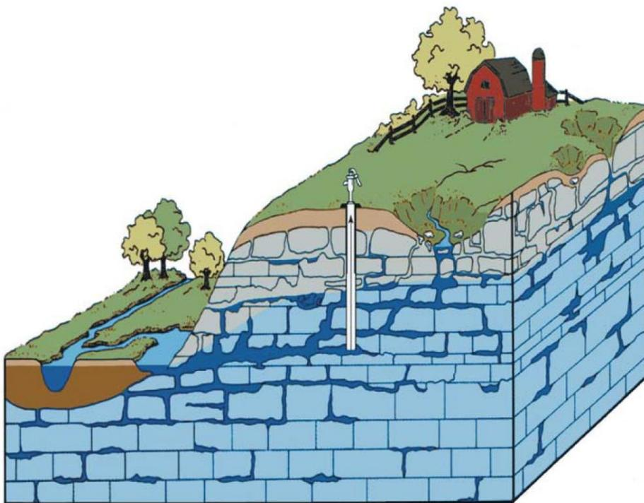
**Figure 1.** A diagram of a karst system with sinkholes, fractures, caves, and springs. The illustration represents the direct connection between the aquifer and land surface, resulting high water yields, and high potential for surface contamination to enter the source aquifer (Hallberg, 1982).
