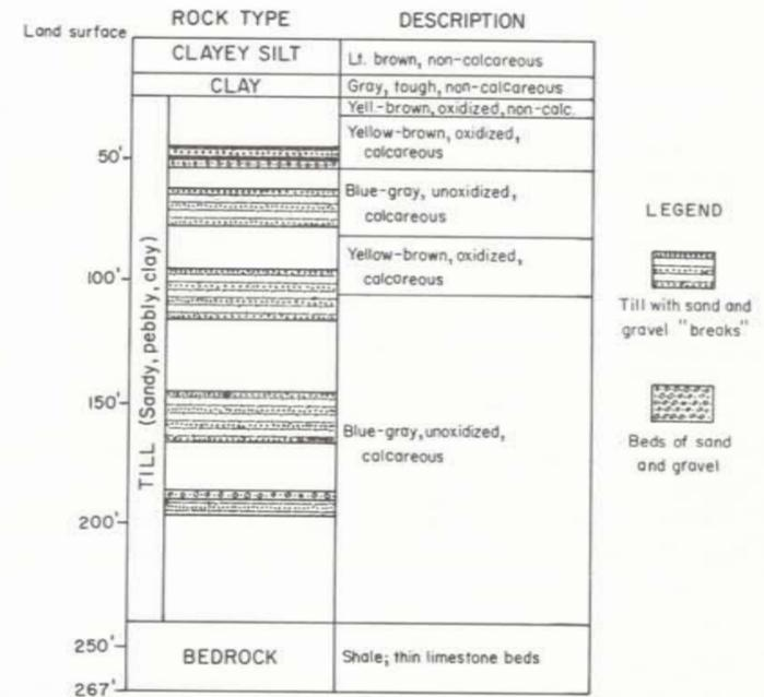
FIGURE 8.—Log of test hole W-51, which is representative of the composition of the glacial drift in the county.
