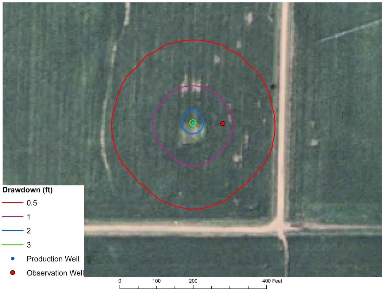
**Figure 11.** ILRW Test Well P-2B pump test simulation results.
