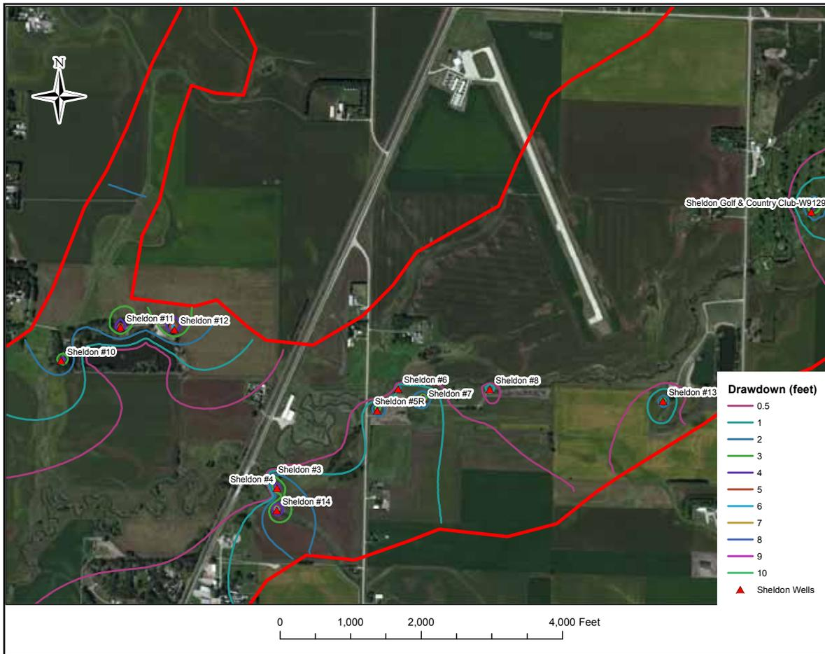
**Figure 12.** Simulated drawdown in feet under severe drought conditions for the Sheldon local scale model.
