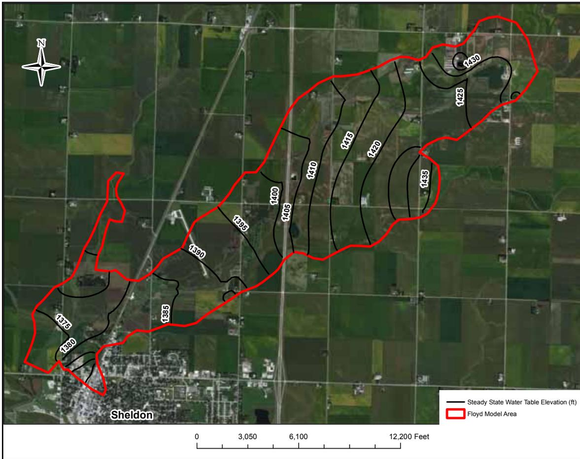
**Figure 10.** Simulated Water Table Elevation under steady-state (non-pumping) conditions for the Sheldon local scale model.
