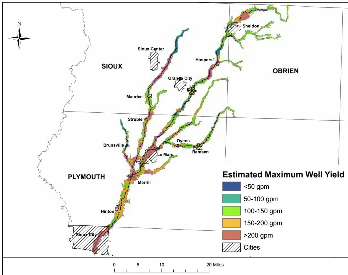
**Figure 9.** Potential well yield in gallons per minute (gpm) based on Figure 8 and available drawdown.
