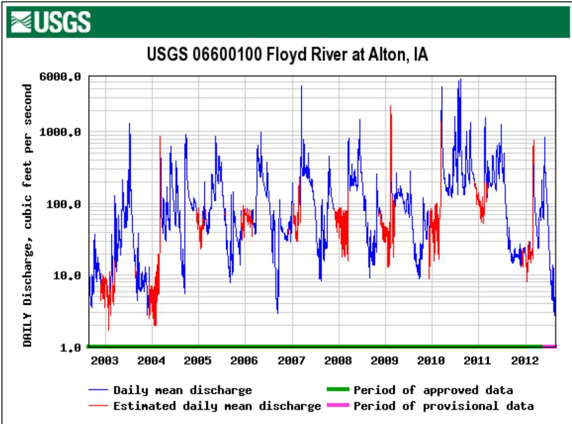
Figure 2. Daily average streamflow at USGS stream gage at Alton (2002 to 2012).
