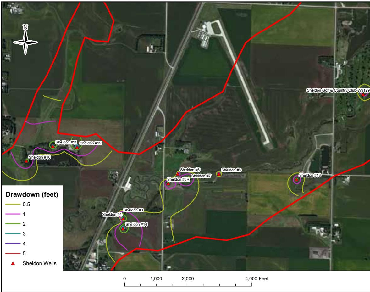
**Figure 11.** Simulated drawdown in feet under normal precipitation conditions for the Sheldon local scale model.
