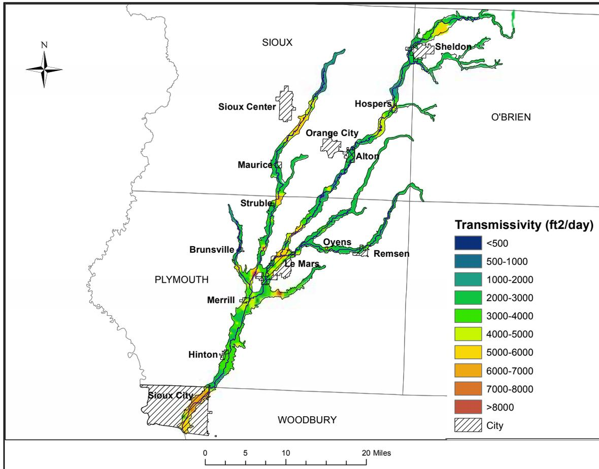
**Figure 8.** Transmissivity distribution within the Floyd River aquifer based on data found in Table 6.
