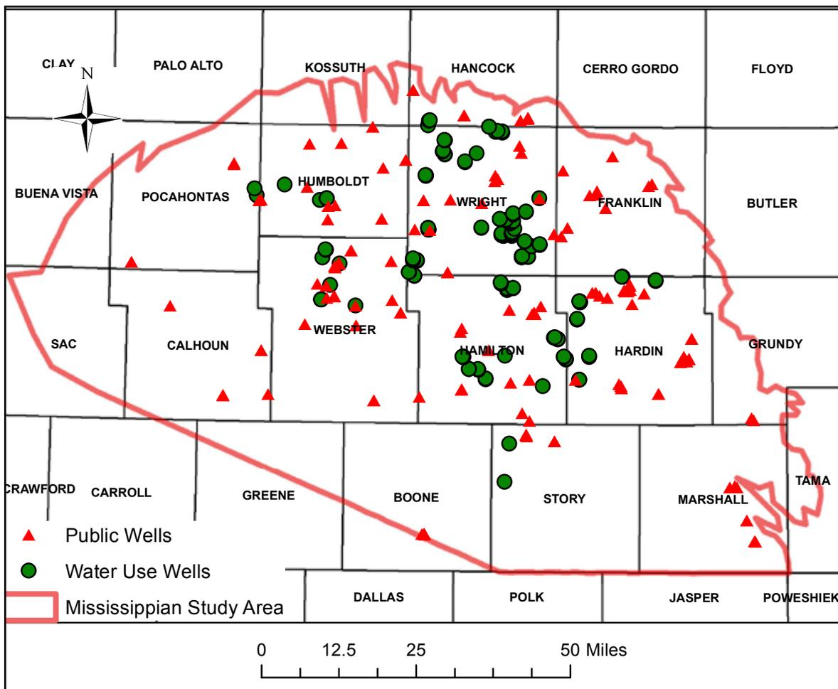
**Figure 8.** Production wells used for transient simulation.
