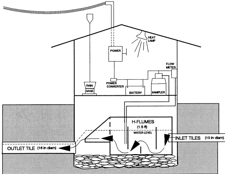
Figure 16. Diagram of the Bughenhagen sub-basin instrument shed.
