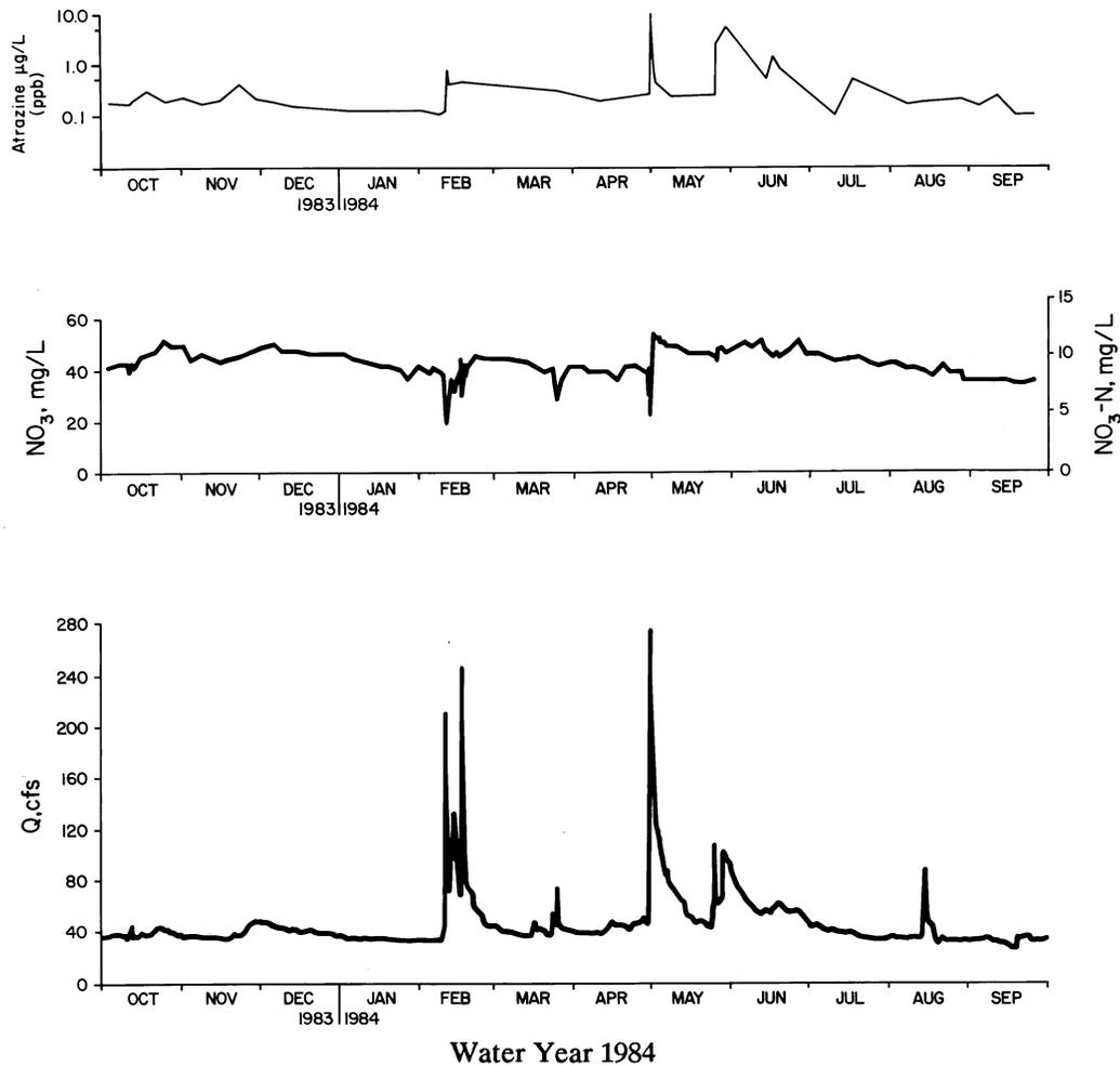
**Figure 21.** Groundwater discharge, and atrazine and nitrate concentrations at Big Spring for WY 1984.
