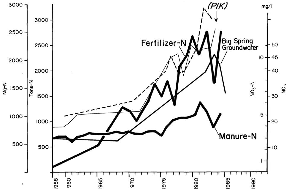
**Figure 25.** Estimated inputs of fertilizer and manure nitrogen to the Big Spring basin and nitrate concentrations at Big Spring, 1958-1985.
