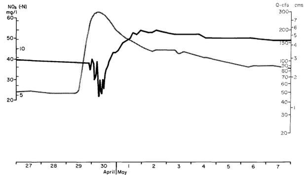
**Figure 23.** Groundwater discharge and nitrate concentrations at Big Spring, April/May 1984.
