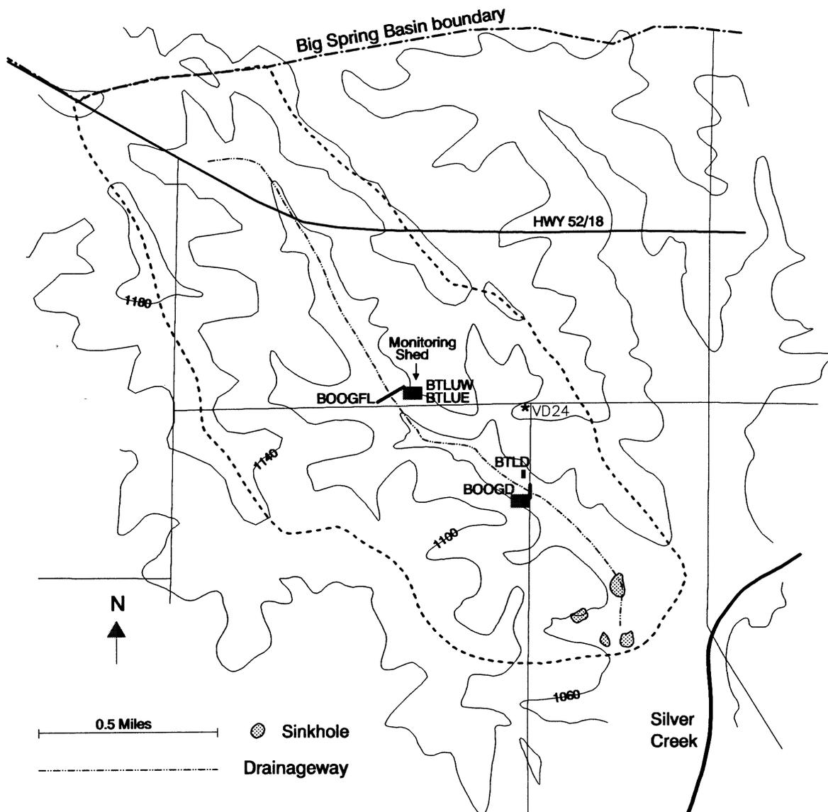
**Figure 15.** Topographic map of the Bugehagen sub-basin showing monitoring site locations.
