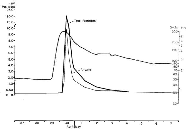
**Figure 22.** Groundwater discharge, and atrazine and total pesticide concentrations at Big Spring, April/May 1984.
