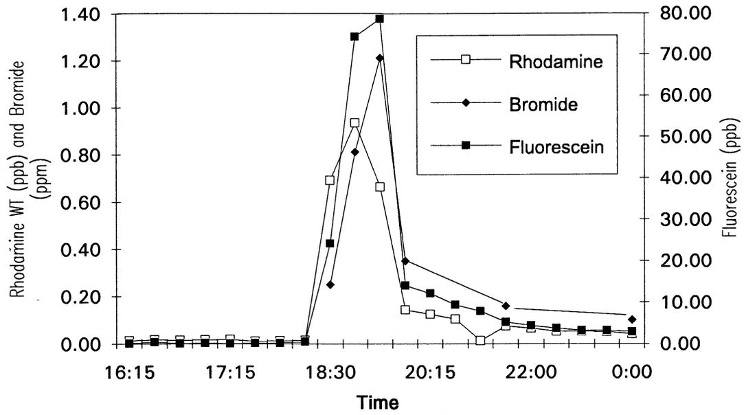
**Figure 18.** Concentrations of tracers in the discharge from L22T during irrigation dye trace, 6/27/90.
