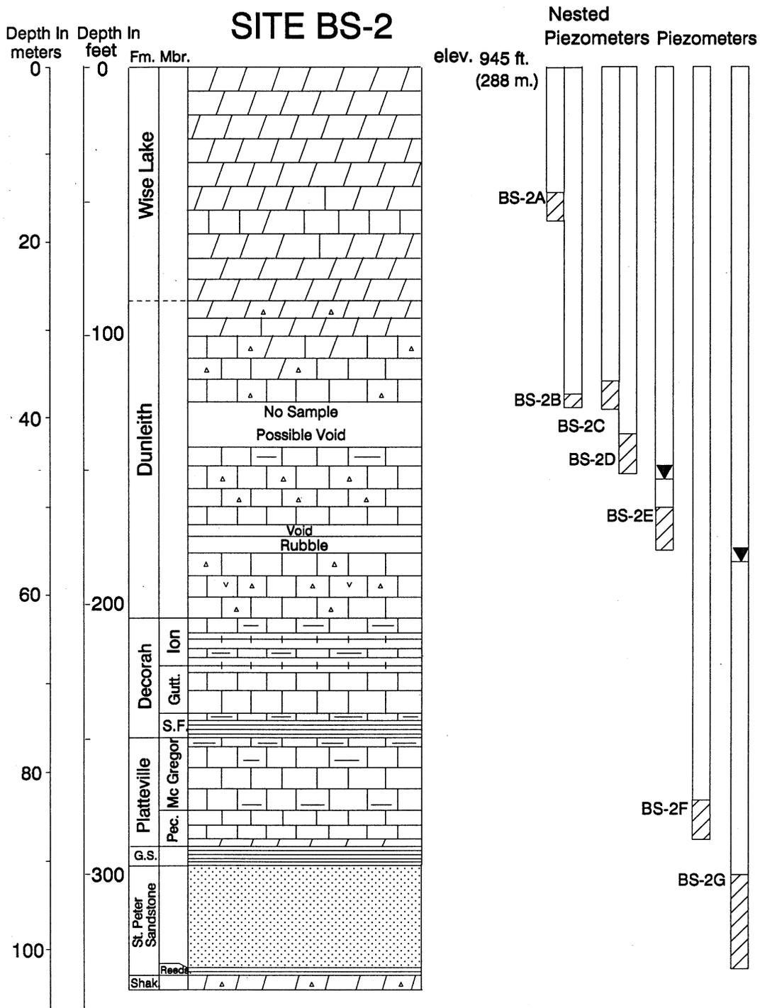
Figure 13. Stratigraphic sequence and monitoring-well installations at Site BS-2 (core logged by M.J. Bounk).
