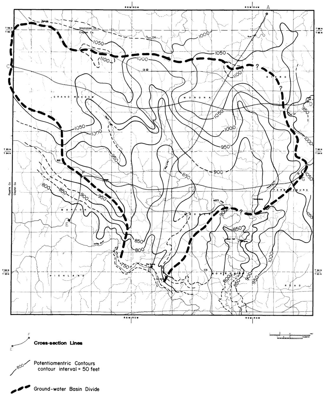
**Figure 7.** Map showing the potentiometric surface of the Galena aquifer. Cross-section lines for Figures 8, 9, and 10 are also shown.
