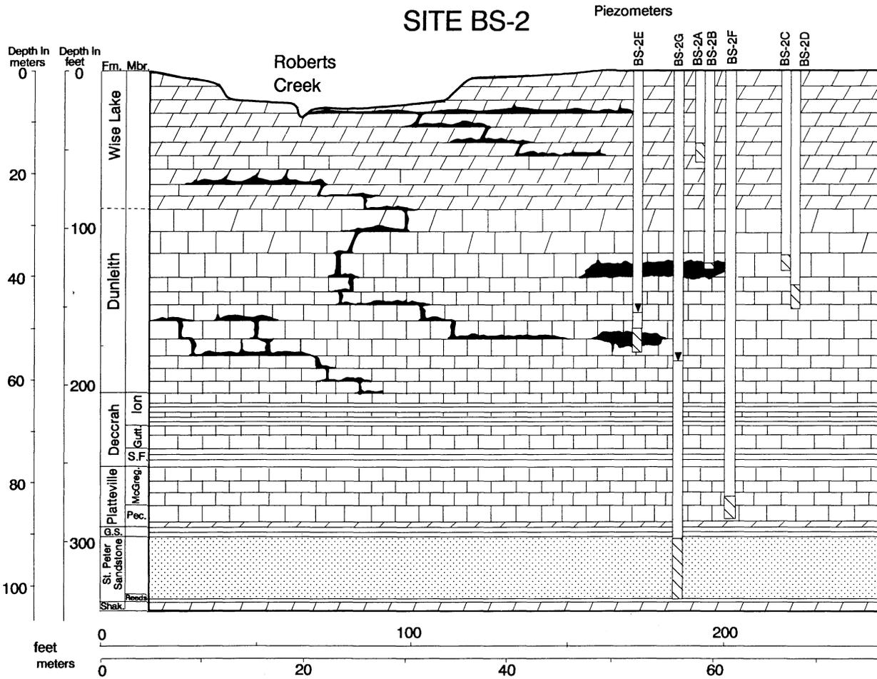
**Figure 14.** Geologic cross-section and monitoring-well installations at site BS-2. Shaded areas represent documented or inferred solution voids and solutionally enlarged fractures and bedding planes.
