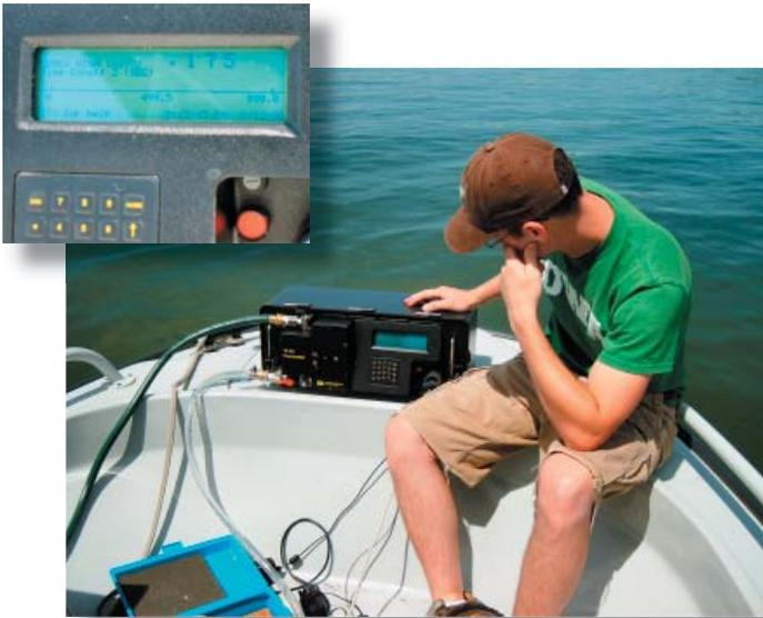
*Sampling for optical brighteners at Clear Lake using the Turner Designs 10-AU Field Fluorometer.*
