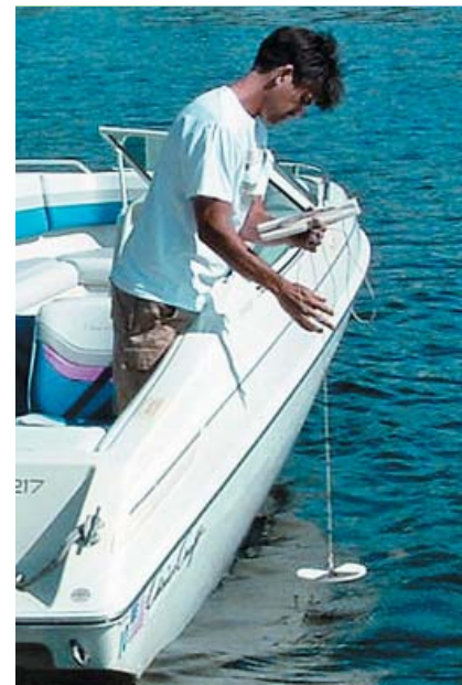
A CLAMP volunteer uses a Secchi disk to measure water clarity.
