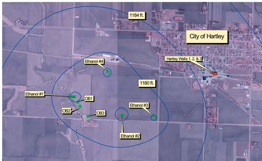
**Figure 6.** Groundwater flow map (potentiometric surface) after 10 years of pumping the proposed ethanol wells. With 10 years of pumping, depression in the potentiometric surface extends beyond the City of Hartley to the northeast.
