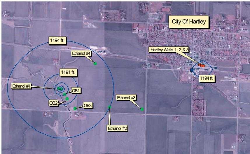
**Figure 5.** Groundwater flow map (potentiometric surface) after 3-day pump test for Hartley, Iowa. A potentiometric surface is an imaginary surface defined by the level to which water will rise in a well. With the 3-day pump test, depression in the potentiometric surface is restricted to the area immediately adjacent to the Ethanol #1 well.
