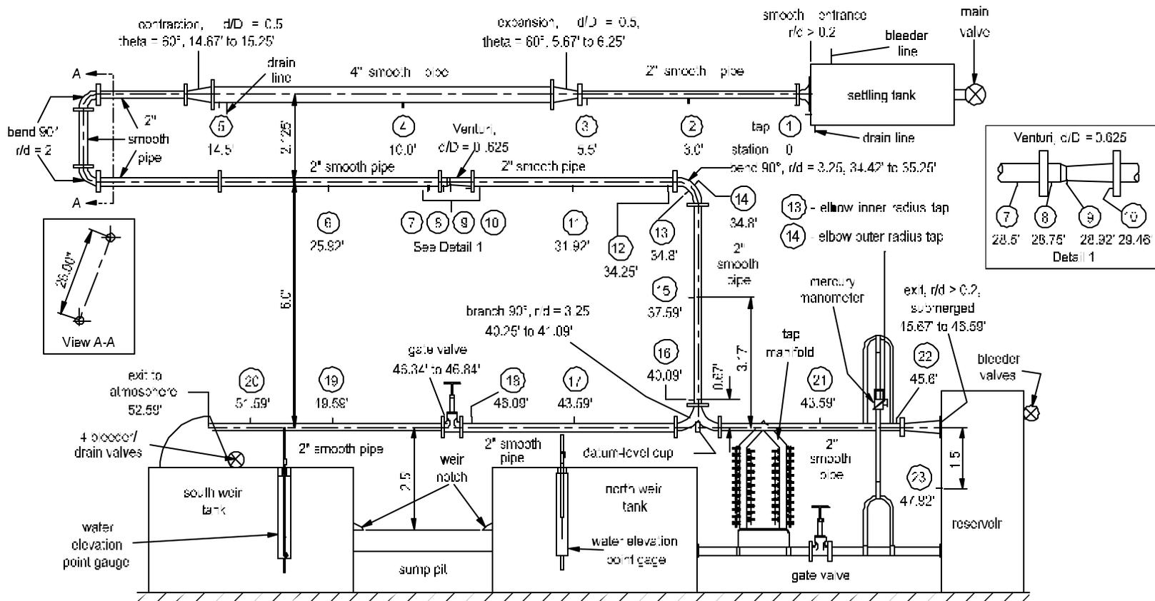
Figure 2.b. The streamlined pipeline assembly
