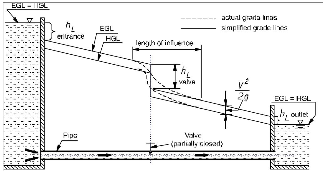
Figure 1. Local head loss through a partially closed vane
