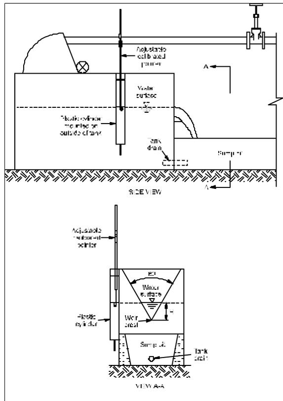
Figure 4. The weir tank and triangular weir
