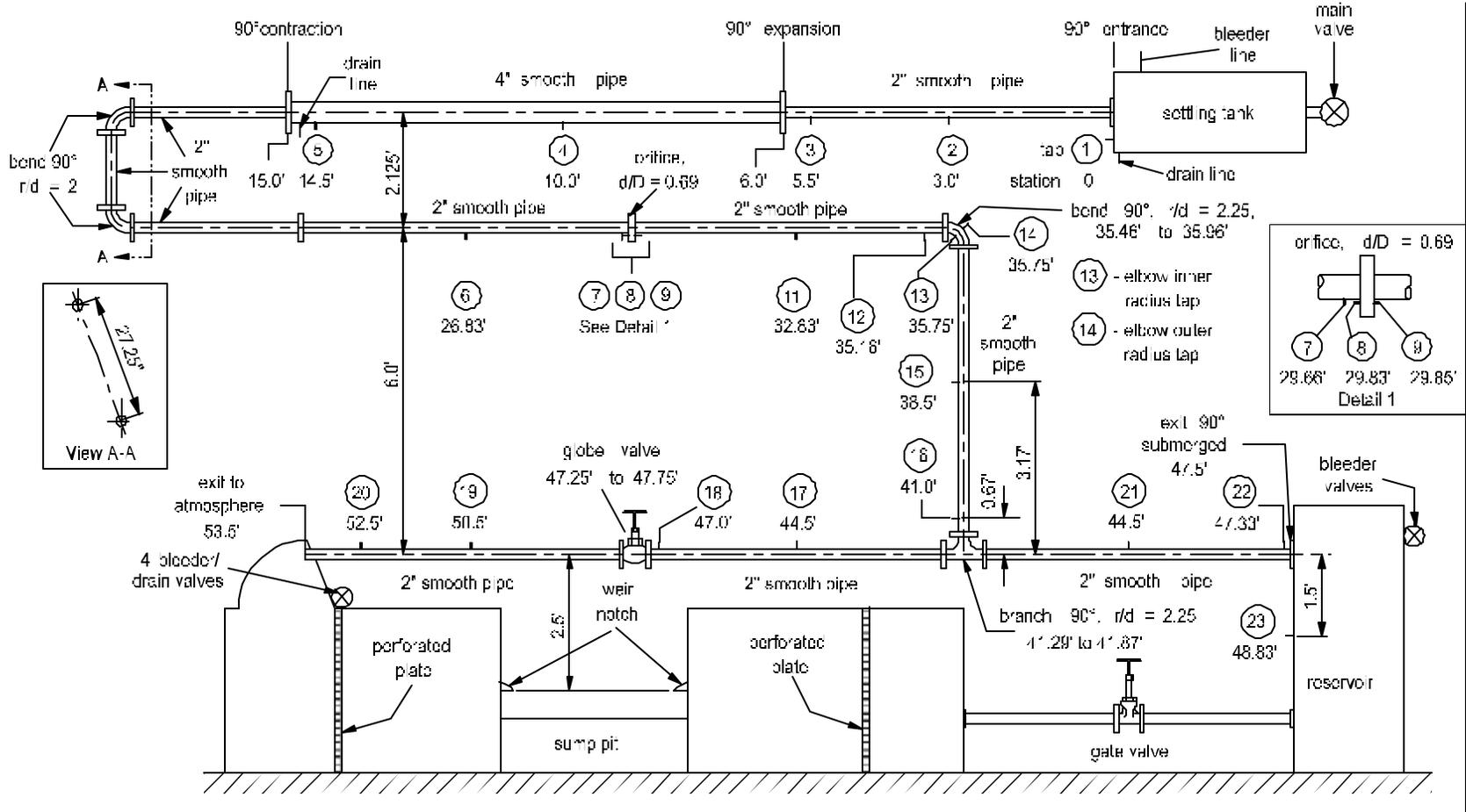
Figure 2.a. The standard pipeline assembly
