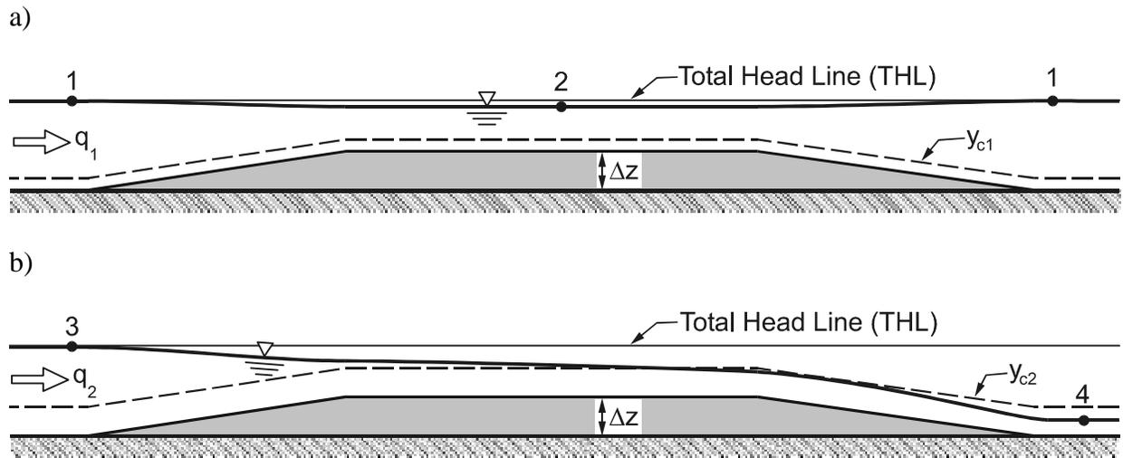
Figure 3. Behavior of the flow over a bump with subcritical flow upstream: a) flow does not attain the critical depth on the bump; b) flow attains critical depth on the bump
