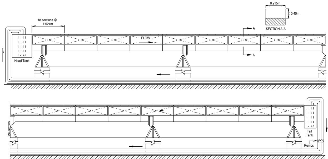
Figure 4. Sketch of the experimental flume
