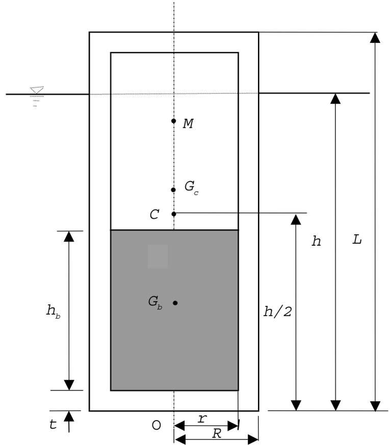
Fig. 2. Hollow cylinder with ballast.
