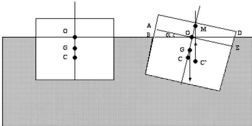
Fig. 1. Metacentric height of a floating body
