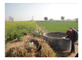
There we waited for Sadiq, Kuldeep, and Zafar, who lead us to various wells throughout the day. Due to time constraints we could not use the Hydrolab so we used the solinst and hach sensor to test water quality. We ran into trouble at the government well where we could not get into the well.
